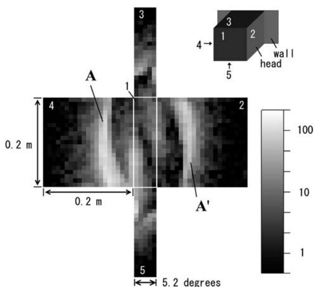
Fig. 3 Strike point pattern on the head for the collisionless regime. The number of the particles is  $2 \times 10^4$ , and 60 % of them are absorbed into the head in this figure. The remaining particles are moving in the configuration space. The regions of the pattern pointed by A and A' are caused by the neo-classical diffusion.
