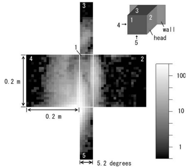
Fig. 2 Strike point pattern on the head for the collisional regime. The number of the particles is  $2 \times 10^4$ , and 55 % of them are absorbed into the head in this figure. The remaining particles are moving in the configuration space. The pattern is not symmetric on the surfaces of the head 2 and 4.
