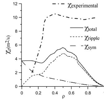
Fig. 7 Neoclassical and experimental electron thermal diffusivities for #32940 LHD shot
