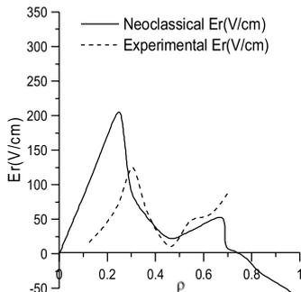
Fig. 6 Neoclassical and experimental electric field ( $E_r$ ) for #32940 LHD shot
