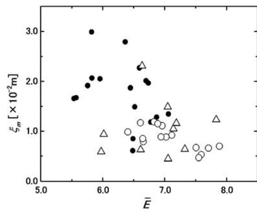
Fig. 4 Elongation dependence of  $n = 1$  mode motions of FRCs with the conducting rings (open circles), the resistive liners (triangles), and without those (closed circles).
