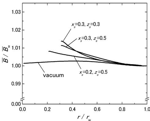
Fig. 2 Radial profiles of averaged magnetic fields calculated from  $z = 0$  to  $z = \ell_s$ .
