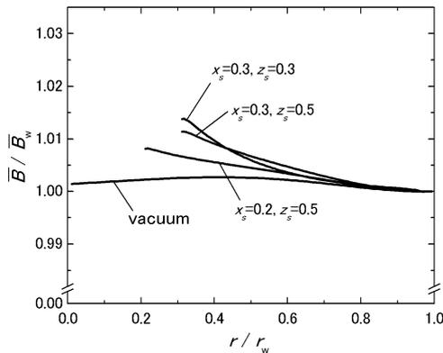
Fig. 2 Radial profiles of averaged magnetic fields calculated from  $z = 0$  to  $z = \ell_s$ .
