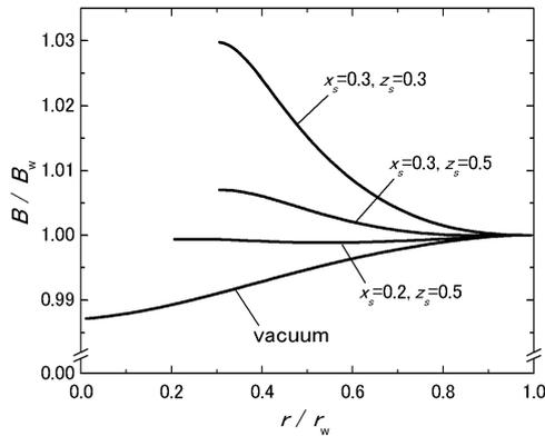
Fig. 1 Radial profiles of magnetic field outside FRCs at the midplane for a mirror coil.
