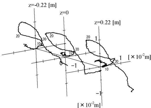
Fig. 3 Trajectories of a plasma column on the  $x$ - $y$  plane at three axial positions, where Arabic numerals denote the time in  $\mu\text{s}$  from a start of the confinement field.
