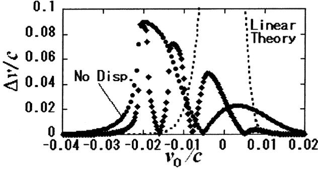
Fig. 2 Perpendicular electron velocity-shifts after interaction with a weakly nonlinear pulse are plotted as a function of  $v_0$ . The perpendicular velocity shifts due to the nondispersive wave packet shown here by squares demonstrate a bifurcation of cyclotron resonance. Other symbols are the same as in Fig. 1.
