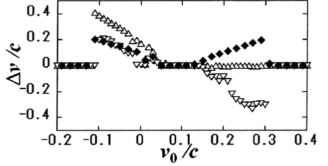
Fig. 3 Parallel and perpendicular electron velocity-shifts due to a nonlinear pulse are plotted as a function of  $v_0$ . Parallel accelerations are generally stronger than perpendicular ones
