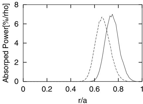
Fig. 4 Calculated absorption profiles with (solid line) and without (dotted line) scattering.
