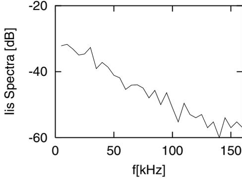
Fig. 1 Spectra of ion saturation current measured at the edge of plasmas.
