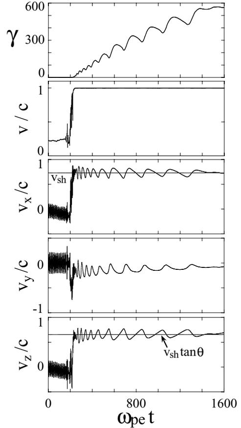
Fig. 3 Time variations of  $\gamma$ ,  $v$ ,  $v_x$ ,  $v_y$ , and  $v_z$  of an accelerated positron.
