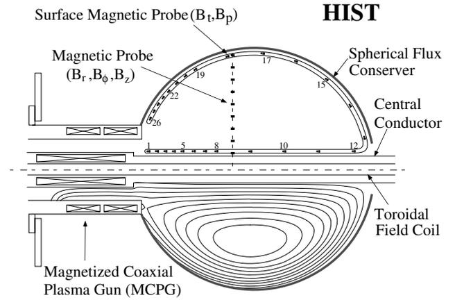
Fig. 2 The schematic drawing of the HIST device and diagnostics.
