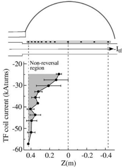
Fig. 4 Dependence of the axial length  $Z$  of the non-flipped (non-reversal) region on the reversed-TF coil current  $-I_{tf}$ .
