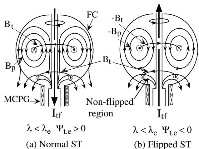
Fig. 1 Comparison of poloidal flux topologies between two kinds of relaxed states (ST (a) and F-ST (b)) in driven-toroidal systems which depend on the direction of the external toroidal flux  $\Psi_{t,e}$ .
