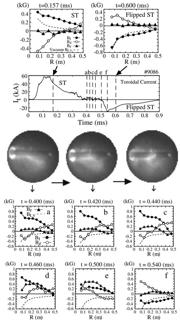
Fig. 3 Time evolution of toroidal current, and the radial profile of magnetic fields of ST, F-ST, and during the transition process from ST to F-ST. Fast framing camera image corresponds to the magnetic field profile of (a, b, c).
