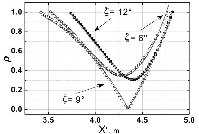
Fig. 2 VMEC data points and analytical fit curves  $\rho(X')$  at  $R_{ax} = 3.6$  m,  $\beta = 0.22\%$  for SDNPA detector #3.
