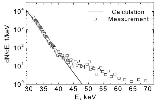
Fig. 3 Calculated (solid) and experimental (dots) atomic energy distribution from  $n_e = 4 \times 10^{13}$  cm<sup>-3</sup> NBI plasma.
