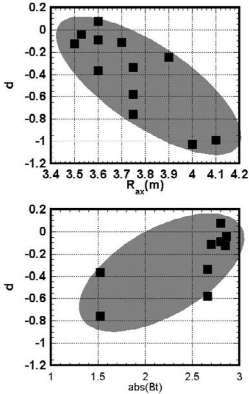
Fig. 4 Magnetic axis dependence (upper) and magnetic field strength dependence (lower). The shadow emphasizes the dependence between  $d$  and magnetic axis/ magnetic field. When the magnetic axis is shifted outward, the dip depth becomes extended due to the large ripple.
