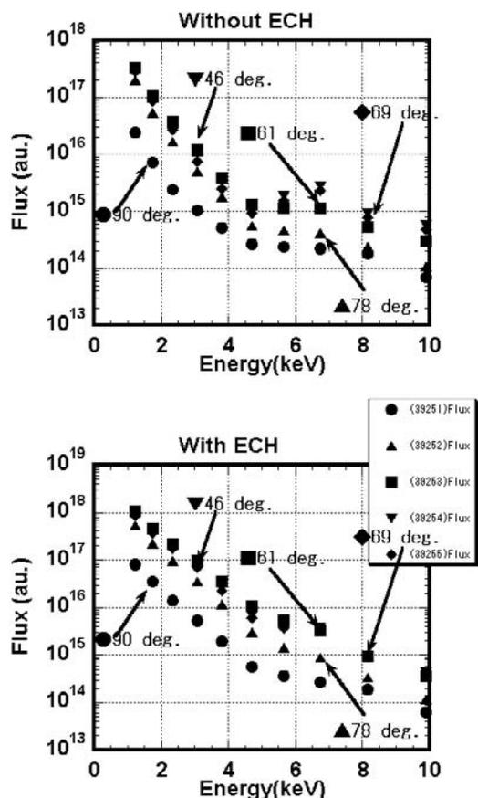
Fig. 1 The spectra without (a)/with (b) ECH. During ECH, the dip around 5 keV disappeared.
