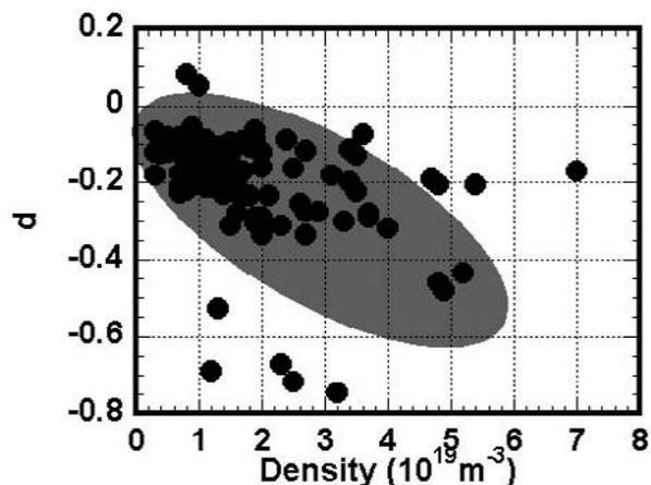
Fig. 2 The density dependence of the dip depth. The shadow emphasizes the dependence between  $d$  and density. Deep dip at high density is due to the negative electric field.
