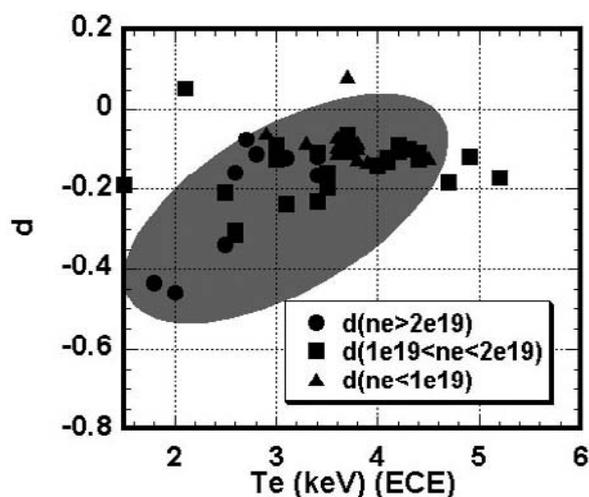
Fig. 3 The temperature dependence of the dip depth. The shadow emphasizes the dependence between  $d$  and temperature. The shallow dip at high temperature is due to the positive electric field.
