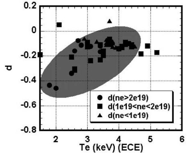
Fig. 3 The temperature dependence of the dip depth. The shadow emphasizes the dependence between  $d$  and temperature. The shallow dip at high temperature is due to the positive electric field.
