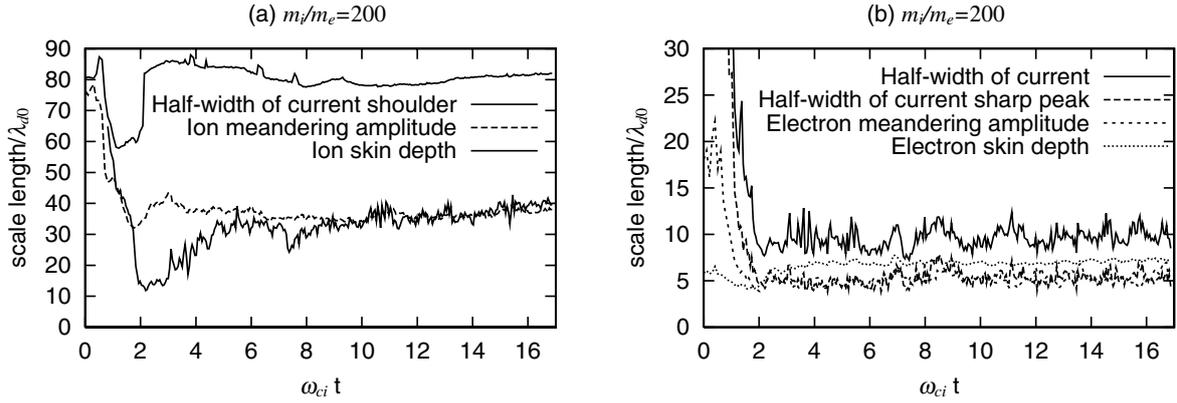
Fig. 2 The time evolutions of several scale lengths: (a) the half-width of the distance of current shoulders, the ion-meandering orbit amplitude  $\lambda_{mi}$  and the ion skin depth  $d_i = c/\omega_{ci}$ , (b) the half-width of a sharp peak of current, the half-width of a current layer, the electron-meandering orbit amplitude  $\lambda_{me}$  and electron skin depth  $d_e = c/\omega_{ce}$ .
