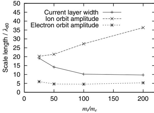
Fig. 3 The mass ratio dependence of scale lengths in the steady state. The half-width of current layer closes to the electron scale for a large mass ratio.
