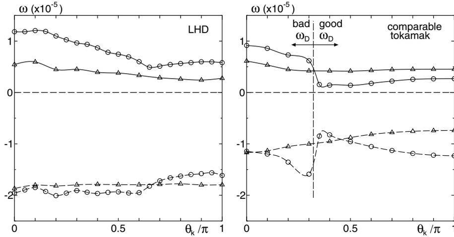
Fig. 4  $\theta_k$  dependence of ITG frequencies in LHD (left) and comparable tokamak (right), at  $s = 0.7$ . Real frequency and growth rate is shown by dashed and solid line with circles. Triangles also show cases that magnetic drift frequency  $\omega_d$  is ignored.
