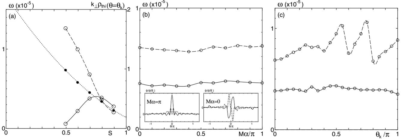
Fig. 6 (a) Radial dependence, (b) field line ( $M\alpha$ ) dependence, (c)  $\theta_k$  dependence of TEM frequencies with  $n_k = 86$ . Solid (dashed) line shows the growth rate (real frequency). Two of local parameters ( $s, \theta_k, M\alpha$ ) = (0.7, 0,  $\pi$ ) are fixed for each dependence plot. In (a),  $k_{\perp}\rho_{thi}(\theta = \theta_k)$  value is also plotted by dotted line on right coordinate.
