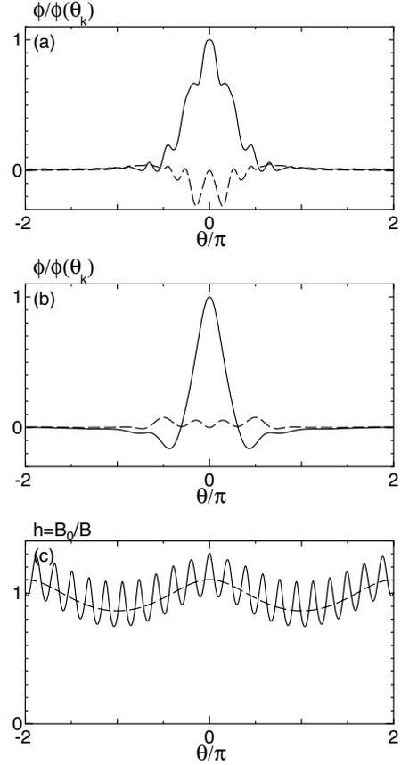
Fig. 3 ITG eigenfunction  $\phi$  for (a) LHD and (b) comparable  $\varepsilon_t$  tokamak, at  $s = 0.7$  and  $k_{\perp}\rho_{thi}(\theta = 0) = 0.6$ . Real (imaginary) part is shown by solid (dashed) line. (c) Modulation of magnetic field strength  $h = B_{\theta}/B$  for the tokamak (dashed line) and LHD (solid line).
