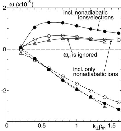
Fig. 1  $k_{\perp}\rho_{thi}$  dependence of ITG frequencies in LHD. Real frequency and growth rate are shown by dashed and solid line respectively. Local parameters are  $(s, \theta_k, M\alpha) = (0.7, 0, \pi)$ . Closed circles are for a case of non-adiabatic ions and electrons, and open circles are for a case of eliminating non-adiabatic electrons. Triangles are for a case of ignoring  $\omega_d$ .
