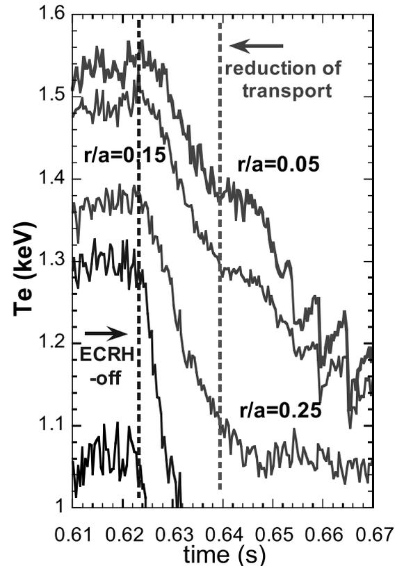
Fig. 2 Interruption of diffusive CPP by abrupt decrease of transport in central zone (observed as disappearance of decay at time shown by second vertical line).
