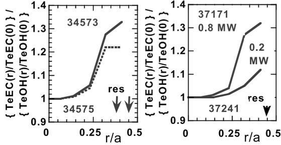
Fig. 3 Comparison of  $T_e$  wideness factor for (a) 0.18MA shots 34573 and 34575 (see Fig. 1(a)). (b) 0.22MA shots 37241 ( $\chi_e^{CP} \approx 0.1 \text{ m}^2/\text{s}$ ) and 37171 ( $\chi_e^{CP} \approx 0.25 \text{ m}^2/\text{s}$ ) with different power.
