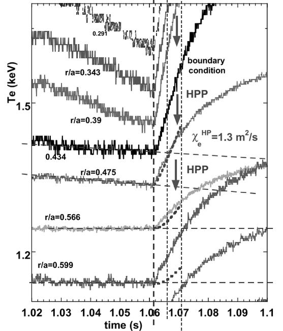
Fig. 5 (a) Profiles of  $|\delta T_e|$  created by ECRH/on-off in LHD shot 28615 (after 4.5ms) - bold and thin solid lines, same by ECRH-on in shot 28614 is shown by dashed curve. (b) Example of HPP, dotted line -calculations.
