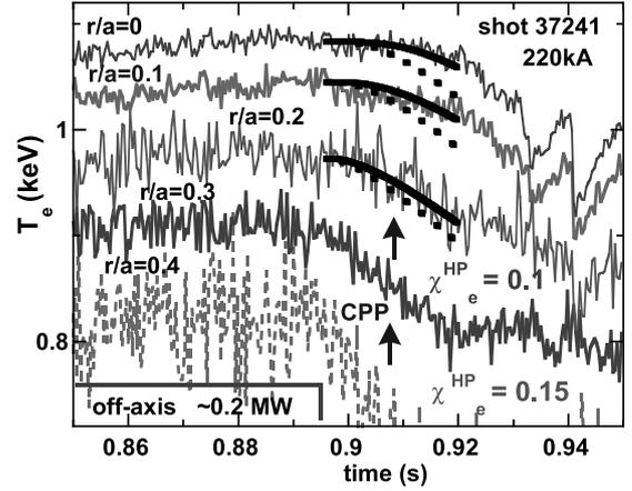
Fig. 4 CPP at 0.22MA/2.33T,  $\bar{n}_e \approx 2.7 \times 10^{19}/\text{m}^3$ , bold and dotted lines represent calculations with  $\chi_e^{CP} = 0.1 \text{ m}^2/\text{s}$  and  $0.2 \text{ m}^2/\text{s}$ .
