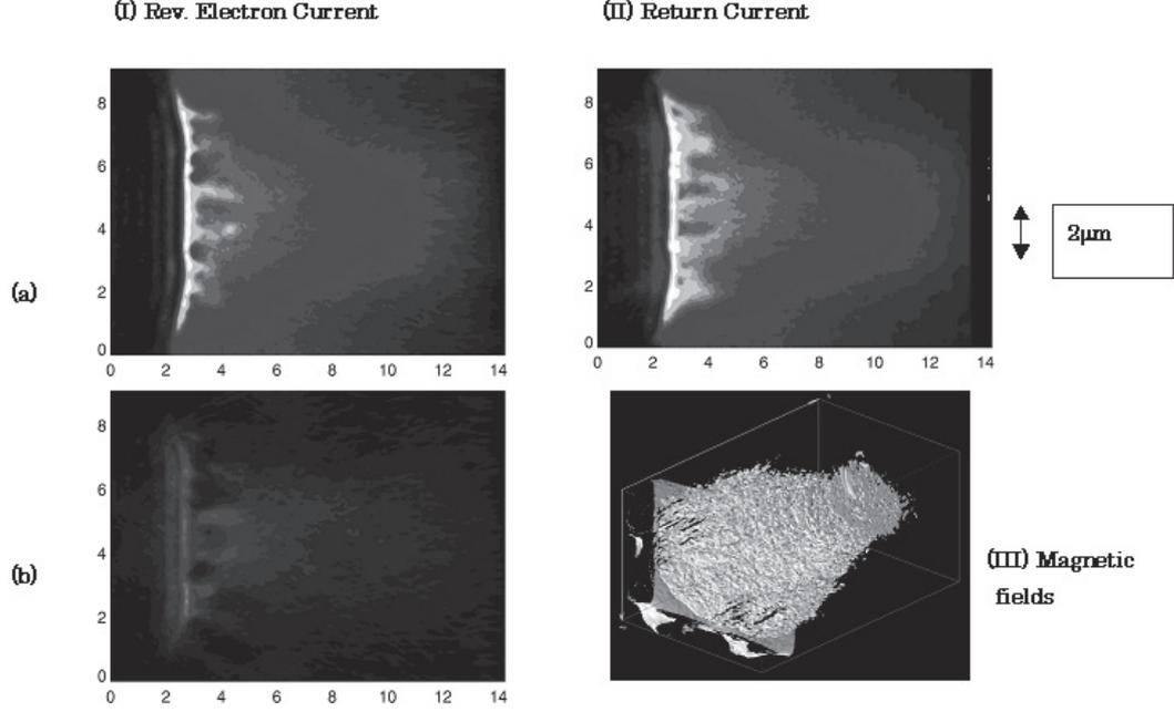
Fig. 2 Relativistic electron current self-organization (self-pinch); (B); (I)–(a); the current profile of hot electron with energy lower than 1.0 MeV, (I)–(b); current profile of hot electron of the energy higher than 1 MeV, (II); return current profile, and (III); magnetic field iso-intensity contour [3].
