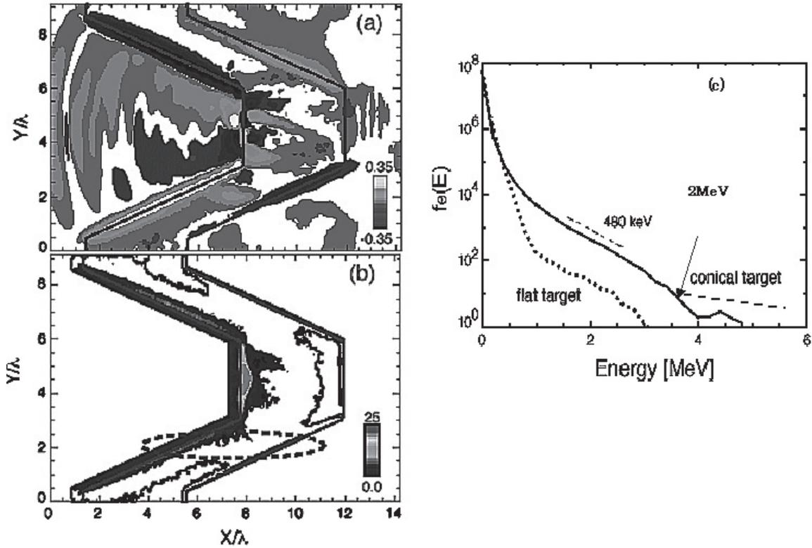
Fig. 4 3D PIC simulation of cone target plasma interactions, (a) contour of magnetic field associated with hot electron flow, (b) contour of hot electron energy density;  $(\gamma-1)n_e/n_c$ , (c) hot electron energy spectrum for cone target and flat target. 480 keV slope temperature electron component is significantly enhanced in the cone.
