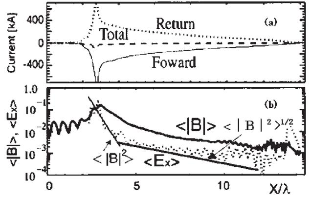
Fig. 3 (a) The spatial profiles of the high energy electron current (Forward) and cold back ground electron current (Return) (b)  $B$  and  $E$  field profiles and phenomenological relation of  $E$  field to  $B$  field.
