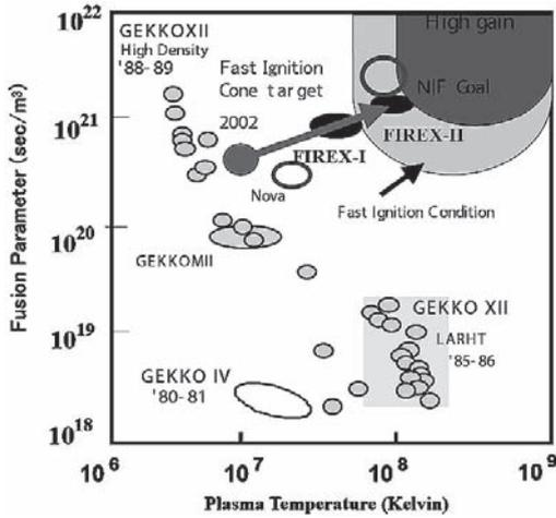
Fig. 6 Fusion parameter achievement by Gekko lasers and NOVA. Ignition condition for fast ignition, FIREX-I and -II, and NIF goals are indicated.
