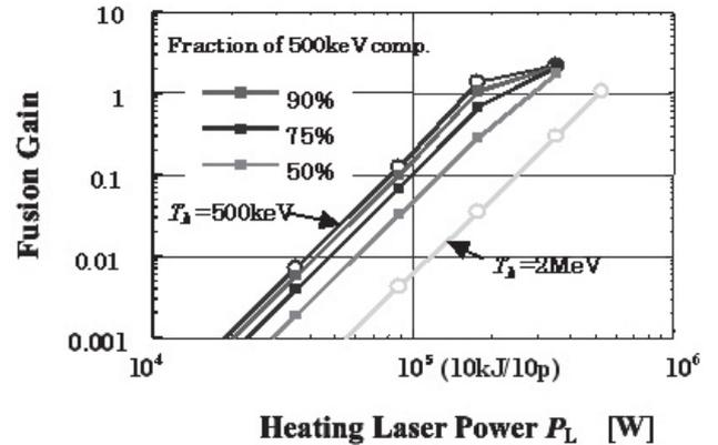
Fig. 5 Fast ignition burning simulation with Fokker Planck transport model. Gain curves for FIREX-I ( $\rho R = 0.7 \text{ g/cm}^2$ ). For the small  $\rho R$ , the fusion gain during the laser heating is significant without ignition. The gain is sensitive to the fraction of low energy relativistic electron component.
