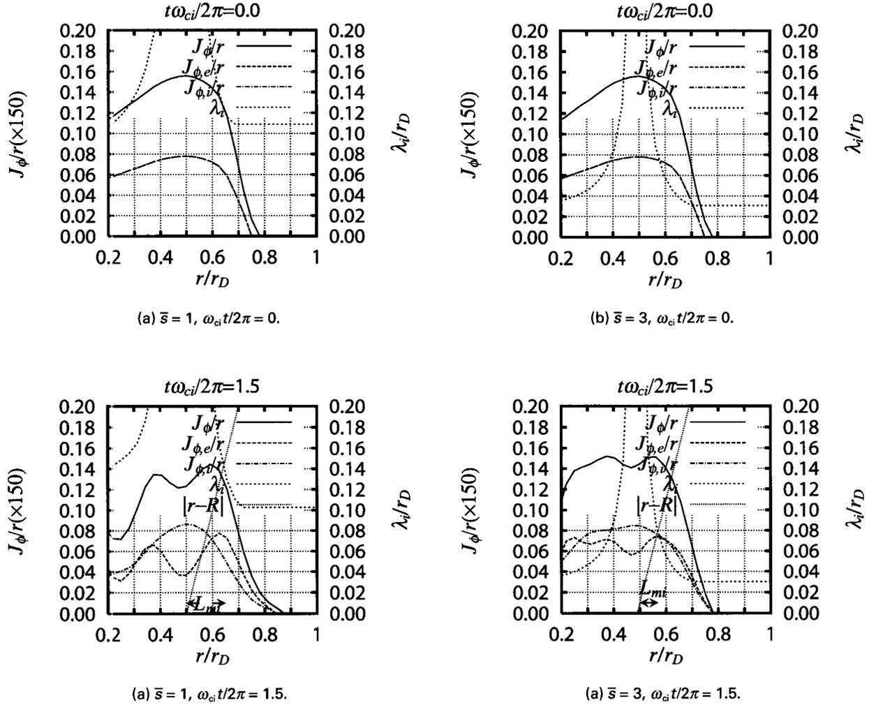
Fig. 4 Current distribution in the radial direction for  $\bar{s} = 1$  and 3 at  $\omega_{ci}t = 0$  and  $3\pi$ . The solid line shows the total current ( $J_{\phi}/r$ ), the broken line shows the electron current ( $J_{\phi,e}/r$ ), the dashed-and-dotted line shows the ion current ( $J_{\phi,i}/r$ ), respectively. The dashed line shows the local ion Larmor radius ( $\lambda_i(r)$ ), and the dotted line shows the distance from the null point ( $|r - R|$ ), respectively.
