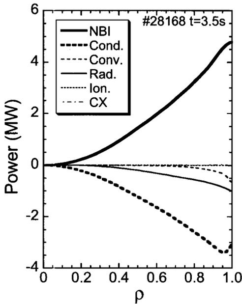
Fig. 3 Power balance at 3.5 s in the discharge illustrated in Fig.2. Input heating power is due to NBI. The major loss channel is conduction. Radiation and convection follow it. Ionization and radiation loss by neutrals (denoted by Ion), and charge exchange loss (denoted by CX) are negligible.
