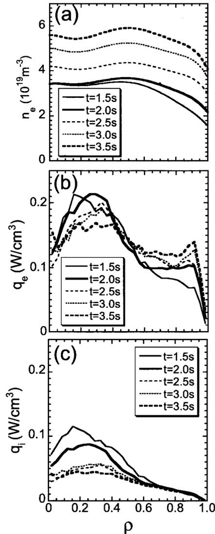
Fig. 4 (a) Electron density and heat deposition profile of NBI power at 5 times of interest in the discharge illustrated in Fig.2. (b) Power deposition to electrons. (c) Power deposition to ions.
