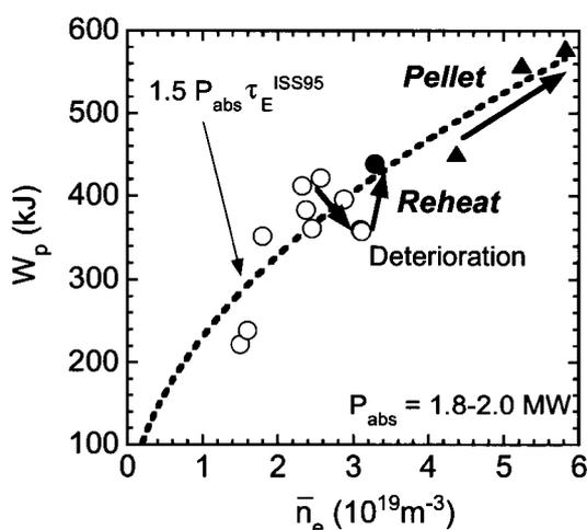
Fig. 1 Dependence of stored energy on line averaged density in the scan with fixed heating power. Open circles: gas-fueled discharge. Solid circle: reheat mode. Solid triangles: pellet-fueled discharge.
