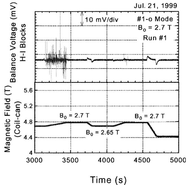
Fig. 1 Typical example of the (H-I) balance voltage signals observed during excitation tests.
