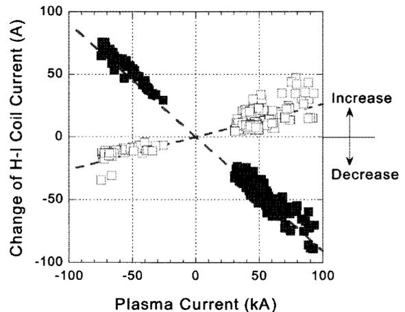
Fig. 3 Relationship between the change of the H-I coil current and the amount of the toroidal plasma current.
