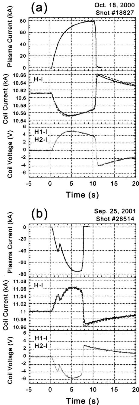
Fig. 2 Waveforms of the toroidal plasma current, the coil current and the terminal voltages of the innermost blocks (H-I) when the toroidal plasma current is induced in (a) the positive and (b) negative directions. The two helical coils (H1 and H2) are connected in series and the current is common. The terminal voltages for the two blocks (H1-I and H2-I) are separately measured.
