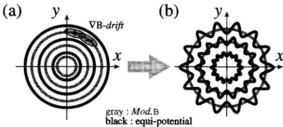
Fig. 1 Schematic diagram of equi-potential surfaces in an axisymmetric mirror, and mechanism of generating the high- $m$  modes on equi-potential surfaces.
