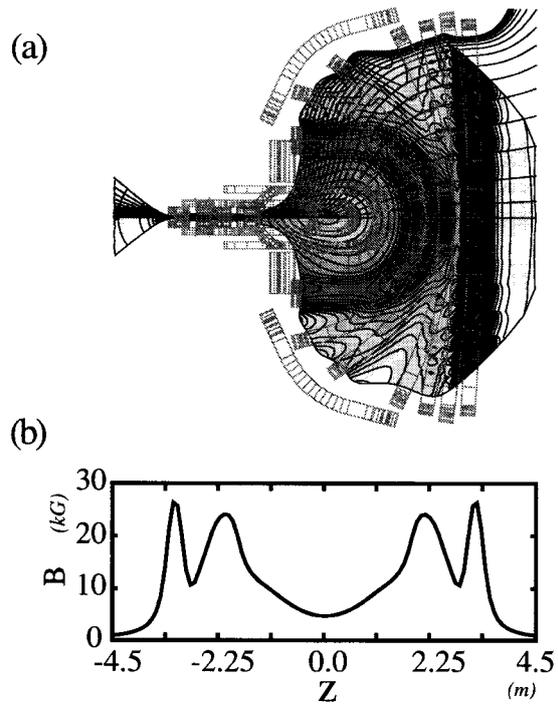
Fig. 6 Magnetic field configuration. (a) is magnetic field lines and contours of magnitude of magnetic field in each component of linked minimum  $B$  mirror coils. (b) is the magnetic field on axis.
