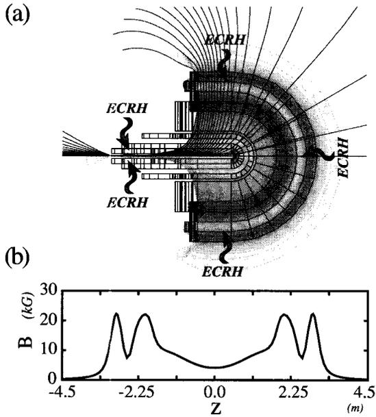
Fig. 3 Magnetic field configuration. (a) is magnetic field lines and contours of magnitude of magnetic field. (b) is the magnetic field on axis.
