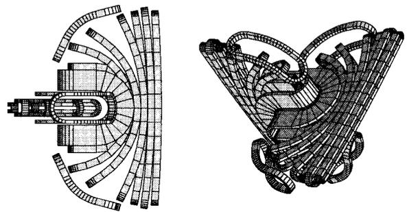
Fig. 5 Schematic diagram of each component of linked minimum  $B$  mirror coils, left figure is a top view and right figure is bird's eye view.
