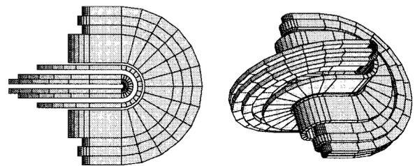
Fig. 2 Schematic diagram of single minimum  $B$  tandem mirror coils, where left figure is a top view and right figure is bird's eye view.
