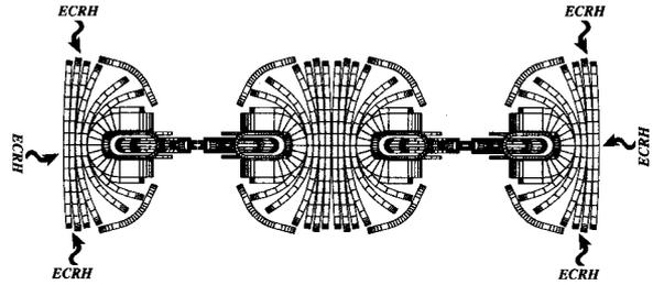
Fig. 4 Schematic diagram of linked minimum  $B$  mirror coils.
