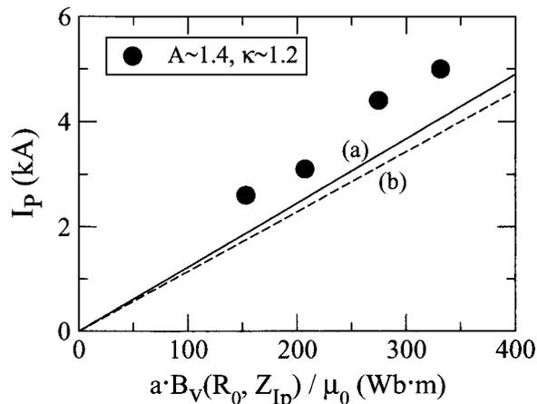
Fig. 6 Observed plasma currents are plotted as a function of the vertical field at the current center. Solid line (a) shows a possible equilibrium vertical field for  $A = 1.4$ ,  $\kappa = 1.74$ ,  $\delta = 0.411$ , and  $R'_0(a) = -0.678$  in ref. [7]. Dashed line (b) shows the vertical field which satisfy the force balance with a given toroidal plasma with  $A = 1.4$  and  $\kappa = 1.2$ , using a plasma self-inductance and a mutual inductance in ref. [8].
