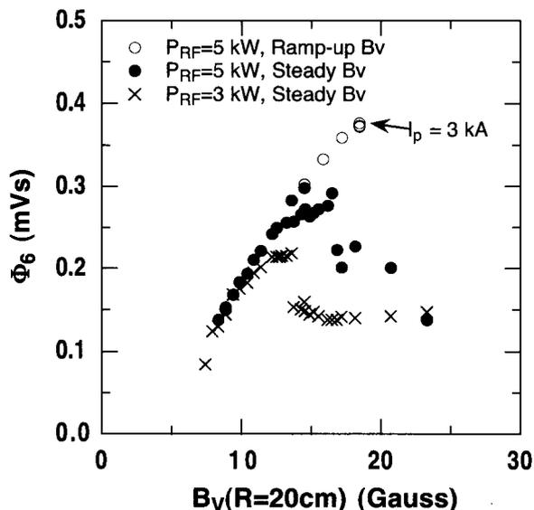
Fig. 4 The flux variation in the No. 6 loop coil versus the vertical field strength.
