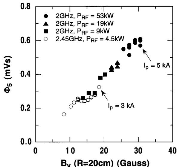
Fig. 5 The flux variation in the No. 5 loop coil versus the vertical field strength for  $P_{RF} = 9, 19, 53$  kW at 2 GHz. Results with 2.45 GHz microwave ( $P_{RF} = 4.5$  kW) are also shown.
