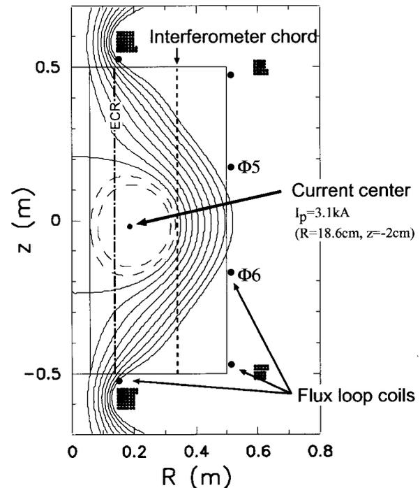
Fig. 2 A contour map of the poloidal flux with  $I_p = 3.1$  kA for the discharge shown in Fig. 1 at  $t = 1.65$  s.
