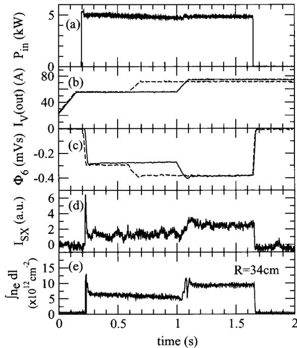
Fig. 1 Time traces of a discharge for  $I_T = 59.4$  kAT,  $P_{RF} = 5$  kW, and  $H_2$  gas pressure  $p_0 = 6 \times 10^{-3}$  Pa. (a) injected microwave power; (b) vertical coil current; (c) flux loop signal  $\Phi_6$ ; (d) soft X-ray emission signal from a SSB diode looking for the whole plasma; (e) line-integrated electron density along the vertical chord at  $R = 34$  cm (see Fig. 2).
