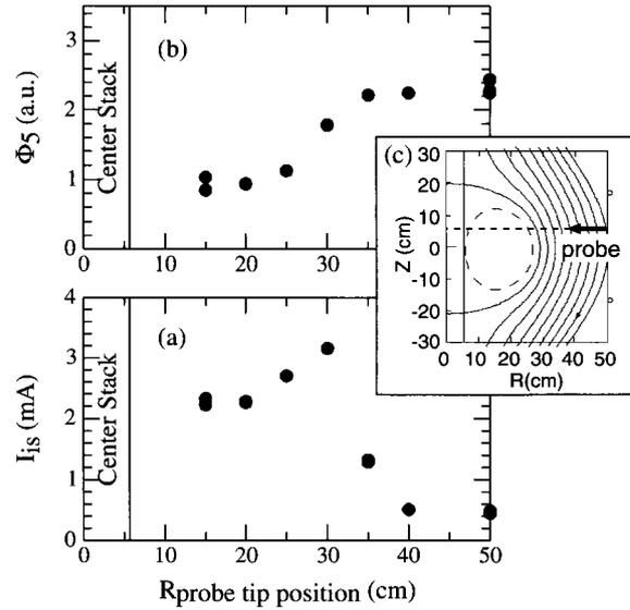
Fig. 3 (a): Radial profile of the ion saturation current at  $z = +6.8$  cm; (b): Flux variation in the No. 5 flux loop coil as a function of the location of the probe tip; (c): Flux contour inferred from the magnetic measurement.
