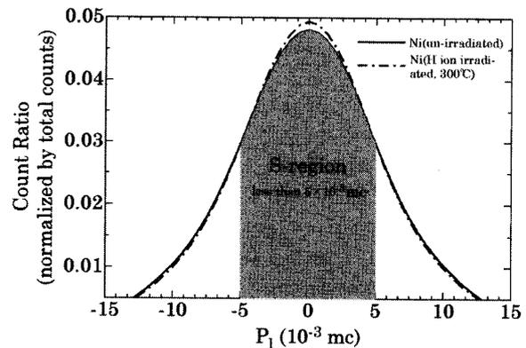
Fig. 3 Comparison of spectra from the CDB measurement between un-irradiated Ni and H ion irradiated Ni at 300°C.
