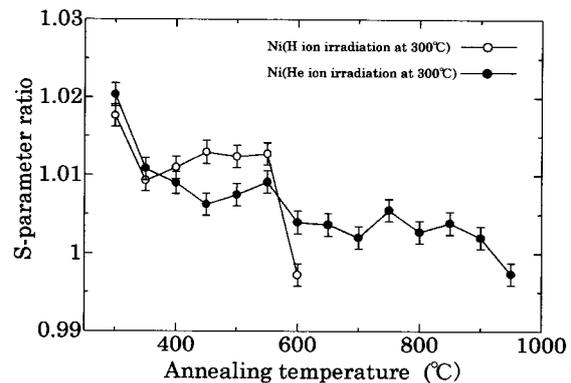
Fig. 4 The isochronal annealing behavior of the S-parameter ratio in Ni irradiated by H and He ions at 300°C.
