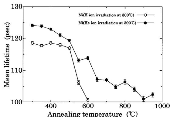
Fig. 2 The isochronal annealing behavior of a mean lifetime component in Ni irradiated by H and He ions at 300°C.
