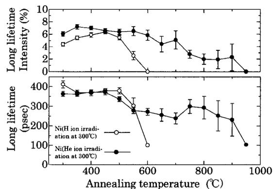
Fig. 1 The isochronal annealing behavior of a long lifetime component and the intensity in Ni irradiated by H and He ions at 300°C.
