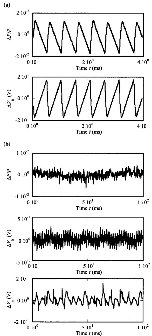
Fig. 1 Time evolution of fluctuations of gyrotron output power  $\Delta P$ , cathode potential  $\Delta V_k$  and anode potential  $\Delta V_a$ . (a) without a smoothing circuit (b) with a smoothing circuit.
