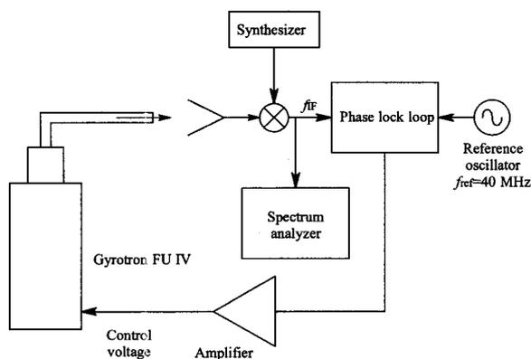
Fig. 3 Block diagram of a phase lock system.
