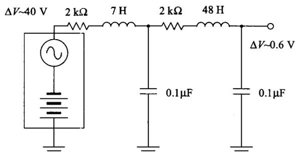
Fig. 2 A smoothing circuit to suppress output voltage fluctuations.
