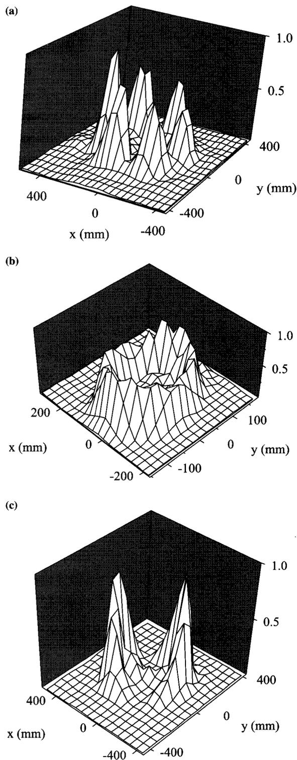
Fig. 7 Intensity profiles of radiation pattern. (a) intensity profile for TE<sub>32</sub> mode ( $B_0=5.5$  T,  $f=151$  GHz,  $z=730$  mm), (b) intensity profile for TE<sub>03</sub> mode ( $B_0=7.0$  T,  $f=194$  GHz,  $z=350$  mm), (c) intensity profile for TE<sub>13</sub> mode ( $B_0=5.8$  T,  $f=163$  GHz,  $z=730$  mm).
