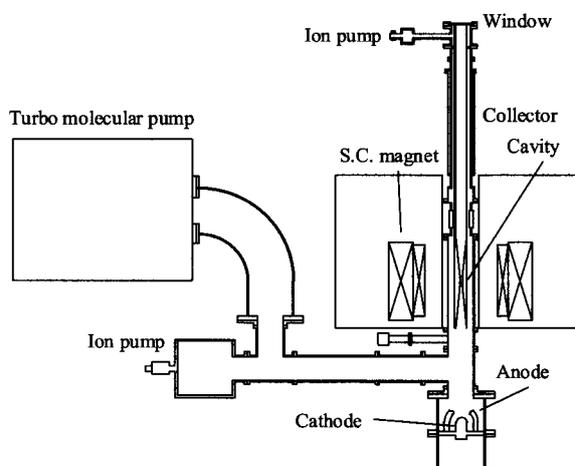
Fig. 5 A schematic drawing of Gyrotron FU VA.
