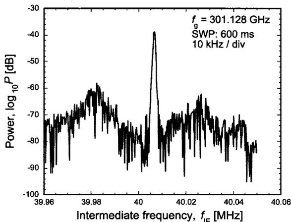
Fig. 4 A logarithmic plot of frequency spectrum of intermediate frequency signal under phase-locked stabilization.
