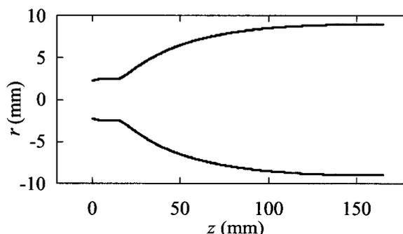
Fig. 6 The shape of the cavity installed in Gyrotron FU VA.
