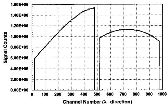
Fig. 2 Relative calibration data using a tungsten lamp (Toshiba, 8V10cd). The left part is the signal frame (0–500 channel) and the right part is the background frame.
