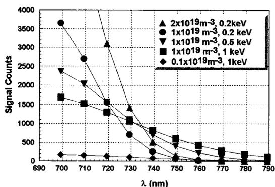
Fig. 3 (b) Estimated Thomson scattering signals for various plasma parameters.
