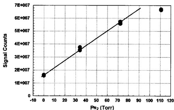
Fig. 3 (a) Rayleigh scattering signals for various nitrogen pressures.
