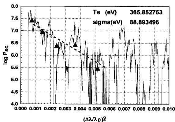
Fig. 4 (b) Electron temperature determined by the calibrated signal. The triangles are averaged values for the 5-nm range. Dashed line shows the fitting for the triangles.
