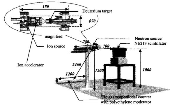
Fig. 1 Structure of a part of accelerator tube and arrangement of experiment.
