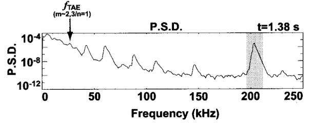
Fig. 5 Power spectrum of magnetic probe signal obtained in LHD. The peak around  $f\sim 200$  kHz corresponds to the high frequency mode. The frequency related to  $m\sim 2+3/n=1$  TAE gap is about 25 kHz.
