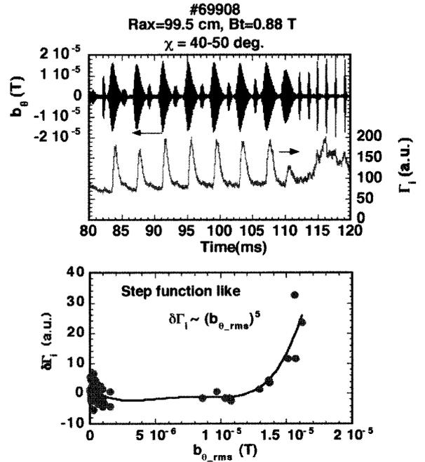
Fig. 6 Time evolution of magnetic fluctuations of  $m\sim 3/n=2$  EPM and energetic ion loss flux measured with a scintillator probe. The lower figure shows the transient increment of the energetic ion loss flux as a function of the EMP amplitude.
