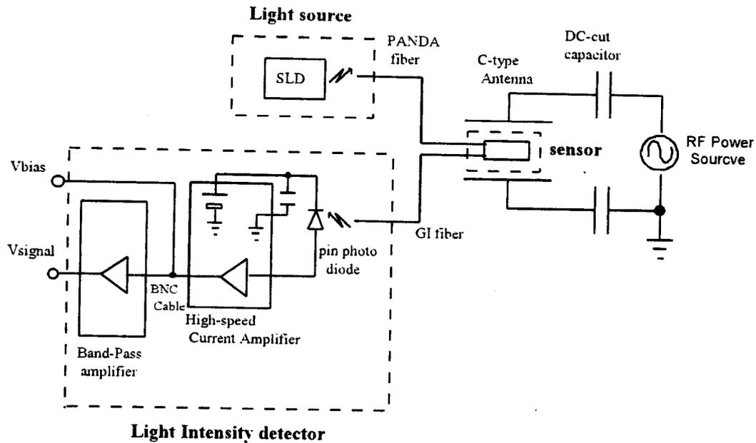
Fig. 1 A schematic diagram of the Pockels probe system. A pair of Pockels cells is used for the sensor.
