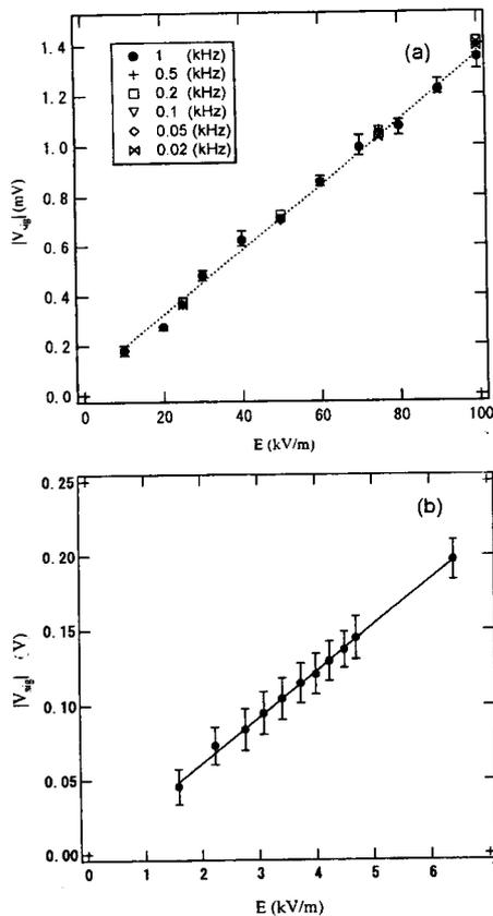
Fig. 4 Plots of the output voltage  $V_{exp}$  at various strengths of oscillating electric fields  $E$ : (a)  $f \sim 0.02$ – $1.0$  kHz (b)  $f \sim 13.56$  MHz. The dotted and solid lines show a least square fitting from the data, which shows that values of  $V_{exp}$  increase linearly with  $E$  as expected.
