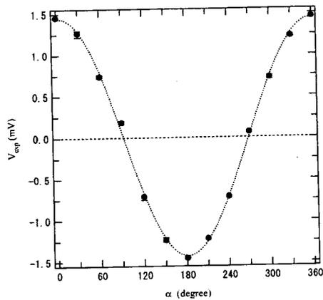
Fig. 3 Plots of  $V_{exp}$  at various angles  $\alpha$  between the Pockels sensor and  $E$ . The plotted data are well fitted by a sinusoidal, showing that the sensor can distinguish the three component of  $E$  in a good resolution.
