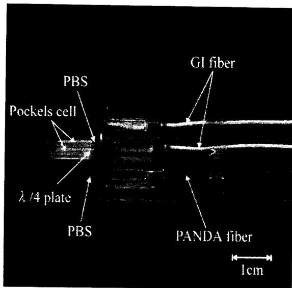
Fig. 2 An enlarged photograph of the sensor indicated in Fig. 1.
