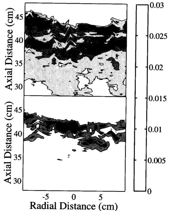
Fig. 2 Two dimensional contour map showing spatial distribution of emitted high energy electrons for incident power of (a) 250kW, (b) 50kW.
