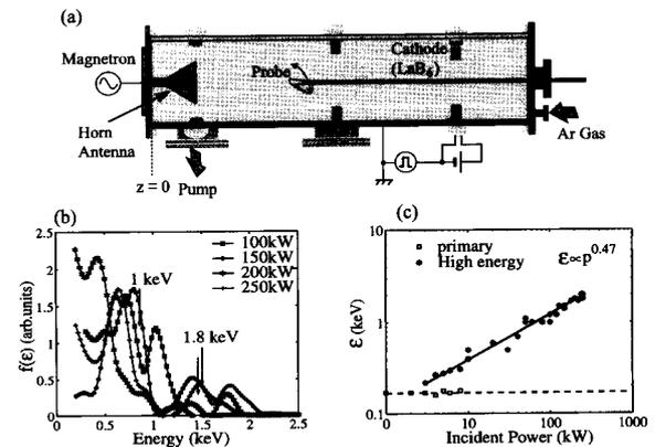
Fig. 1 (a) Experimental setup. (b) Electron energy distribution function for different incident microwave power. (c) Energy scaling law of high energy electrons.
