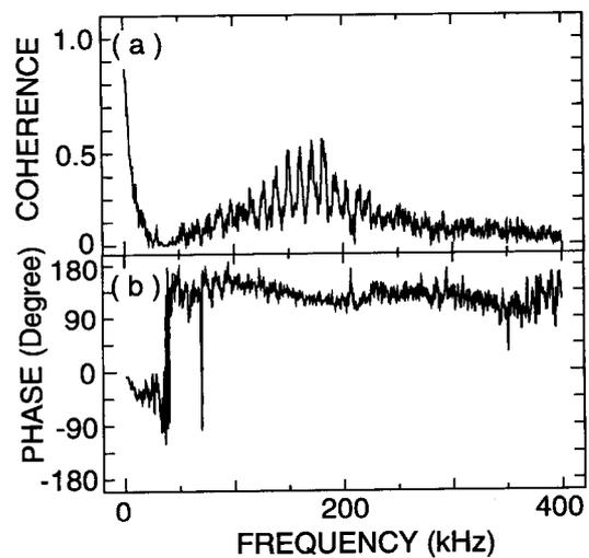
Fig. 4 (a) Cross-correlation function (Coherence) and (b) phase between grid and collector current fluctuations in region I.
