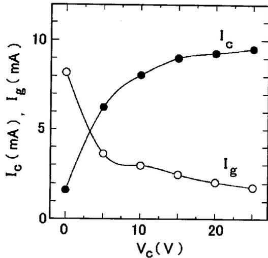
Fig. 5 Dependence of grid  $I_G$  and collector  $I_C$  currents on collector potential  $V_C$ .
