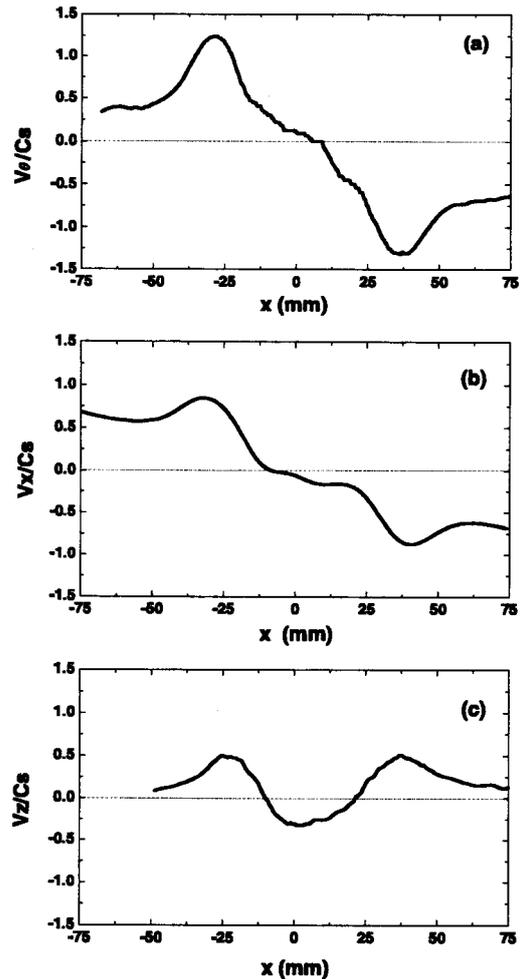
Fig. 5 Velocity profiles of plasma flow measure by DLP at  $z = 1100$  mm with the coefficient  $K = 0.5$ . (a): the azimuthal flow velocity, (b): the radial flow velocity, and (c): the axial flow velocity.
