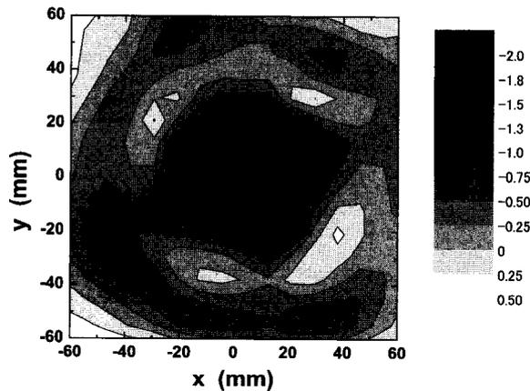
Fig. 6 Vorticity contour on  $z = 1100$  mm plane.
