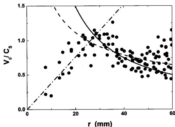
Fig. 7 Azimuthal velocity as a function of the distance from the center of rotation. Dashed line indicates the relation  $V_{\theta} \propto r^{\alpha}$  with  $\alpha = 1$ , solid curve with  $\alpha = -1$ , broken curve with  $\alpha = -0.5$ , respectively.
