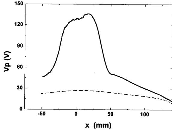
Fig. 4 Plasma potential profile at  $z = 1100$  mm. Solid line indicates the plasma potential in the presence of hole structure under operating condition  $6 \times 10^{-4}$  Torr (He) and 8.5 kW microwave input, dashed line the potential of the uniform plasma under operating condition  $2 \times 10^{-3}$  Torr (He) and 9.6 kW microwave input.
