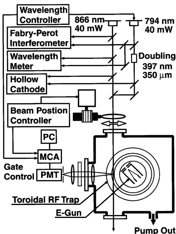
Fig. 1 Experimental setup of the laser-induced fluorescence measurement system.
