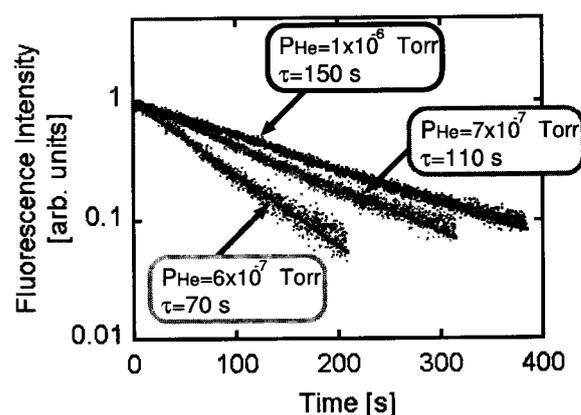
Fig. 3 He gas pressure dependence of the decay of fluorescence intensity of  $Ca^+$ .
