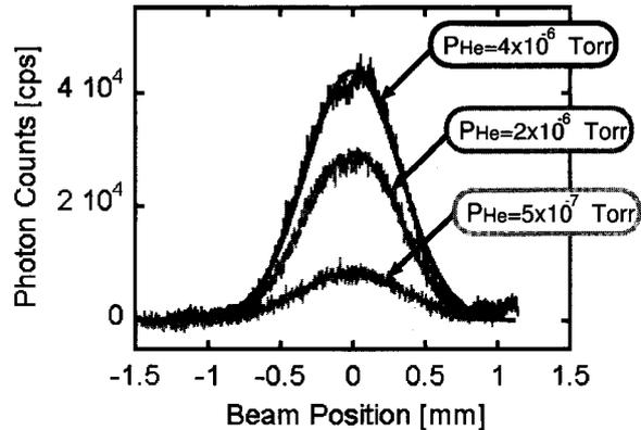
Fig. 5 Helium gas pressure dependence of density profile of the  $\text{Ca}^+$  ion cloud in the poroidal cross-section.
