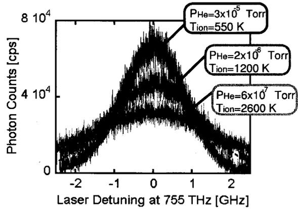
Fig. 4 Helium gas pressure dependence of the Doppler spectrum of the  $\text{Ca}^+$  ion cloud.
