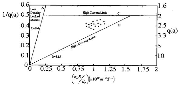
Fig. 2 Hugill diagram showing the boundaries of the IR-T1 operating parameter space.
