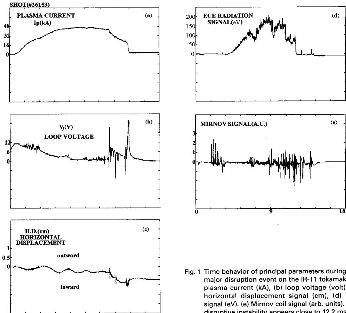
Fig. 1 Time behavior of principal parameters during the major disruption event on the IR-T1 tokamak; (a) plasma current (kA), (b) loop voltage (volt), (c) horizontal displacement signal (cm), (d) ECE signal (eV). (e) Mirnov coil signal (arb. units). The disruptive instability appears close to 12.2 ms.
