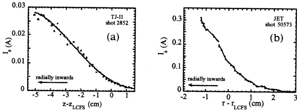
Fig. 2 Radial profile of the ion saturation current (a) in the TJ-II stellarator for a plasma configuration with  $\iota$  (a)  $\approx 1.9$  (i.e. with the 4/2 surface located out of the plasma boundary region) and (b) for the shot 50673 ( $B = 2T$ ,  $I_p = 2MA$ ) in JET.
