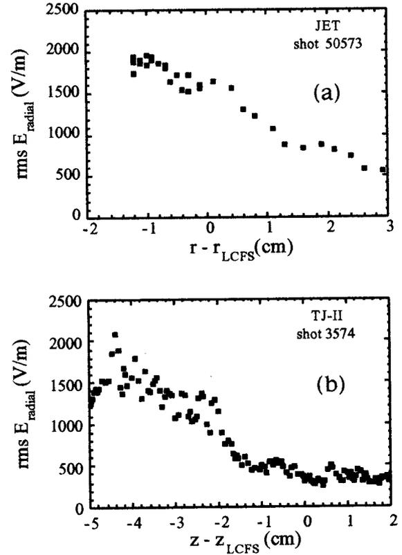
Fig. 4 Root mean square (r.m.s.) value of fluctuations in the radial electric field in the TJ-II stellarator (a) and JET tokamak (b) computed neglecting  $T_e$  fluctuation effects.
