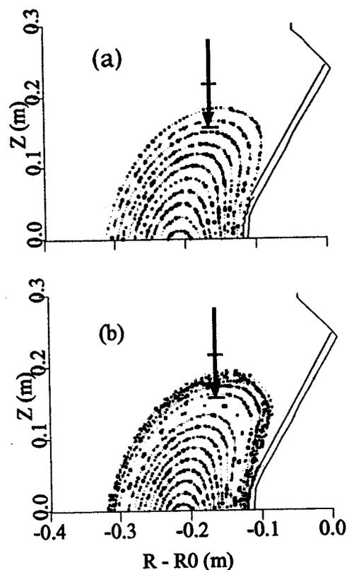
Fig. 1 TJ-II vacuum configuration (a) without and (b) with medium size island ( $n/m = 8/5$ ) in the plasma boundary region.
