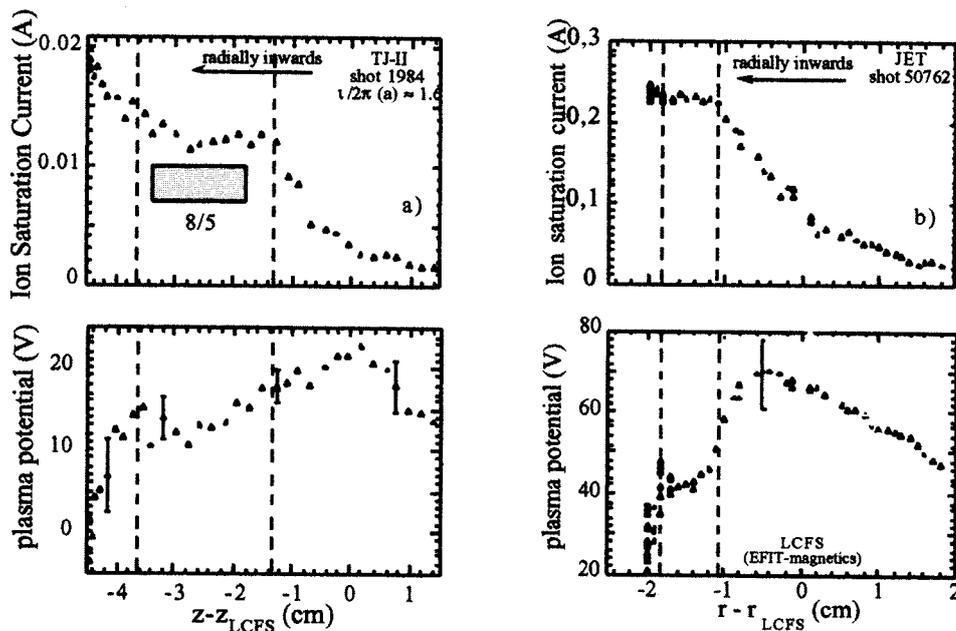
Fig. 3 Radial profiles of the ion saturation current, floating potential and plasma potential (a) in a TJ-II plasma configuration with a low order resonance (8/5) located near the plasma boundary (b) for the JET shot 50762 ( $B = 1T$ ,  $I_p = 1MA$ ).
