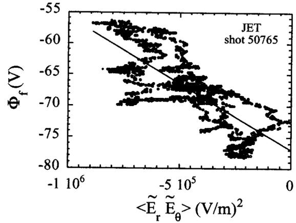
Fig. 5 Correlation between floating potential and the electrostatic Reynolds stress in the plasma edge of JET tokamak.
