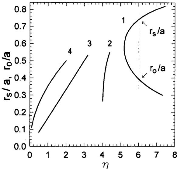
Fig. 2 Separatrix edge radius  $r_s/a$  (and magnetic axis  $r_o/a$  in  $l = 1$  stellarator) as function of  $\eta$  in  $l = 1, 2, 3, 4$  straight stellarators (curves 1-4, respectively).
