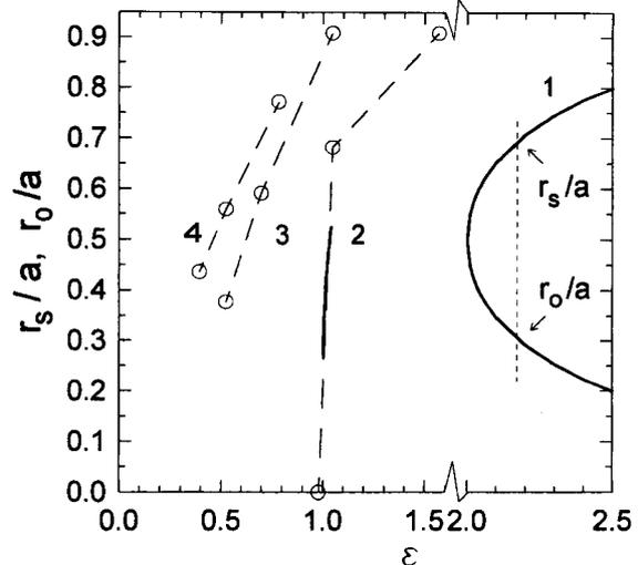
Fig. 3 Separatrix edge radius  $r_s/a$  (and magnetic axis  $r_o/a$  in  $l = 1$  torsatron) as function of  $\epsilon$  in  $l = 1, 2, 3, 4$  straight torsatrons (curves 1-4, respectively).
