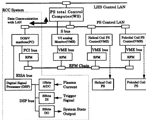
Fig. 2 Structure of the RCC system.
