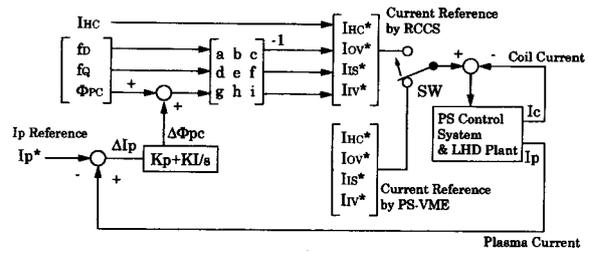
Fig. 3 Block diagram of the coil current feedback system.
