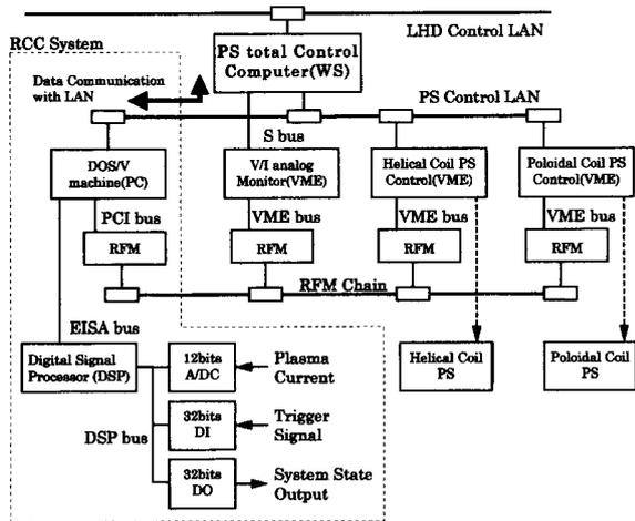
Fig. 2 Structure of the RCC system.
