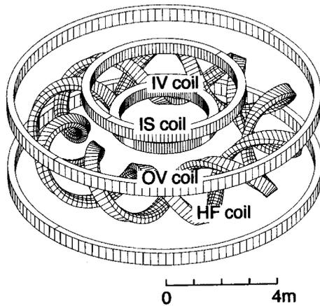
Fig. 1 Schematic of the LHD coil system.
