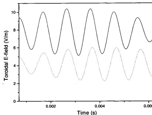
Fig. 6 Toroidal electric field vs. time. Dotted curve estimated from  $v_r \times B_{vert}$  and solid curve from  $V_\phi$ .
