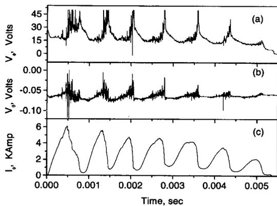
Fig 2. (a) Toroidal loop Voltage ( $V_\phi$ ), (b) Poloidal loop voltage ( $V_\theta$ ) and (c) Plasma current ( $I_p$ ) vs. Time.
