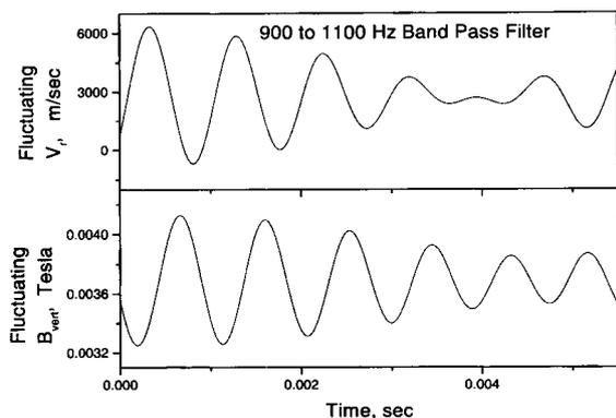
Fig. 5 (a) Fluctuating plasma velocity  $v_r$  and (b) Fluctuating vertical magnetic field  $B_{vert}$  vs. Time.
