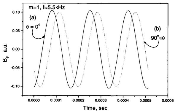
Fig 4. Poloidal magnetic field ( $B_\theta$ ) vs. Time at (a)  $\theta = 0^\circ$  probe and (b)  $\theta = 90^\circ$  probe.
