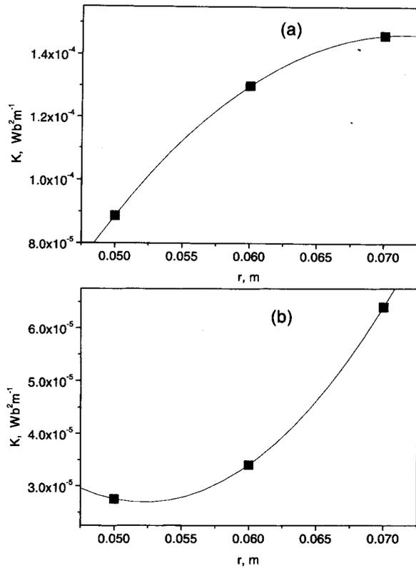
Fig. 3 Helicity ( $K$ ) per unit length vs. Radius ( $r$ ): (a) During peak plasma current, (b) After the crash of plasma current.
