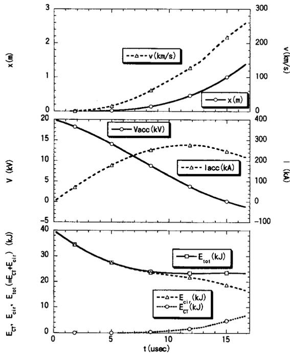
Fig. 1 Simulated waveforms of SPICA mk. I. Point-model [3] is solved using the fourth order Runge-Kutta method. CT mass of 0.2 mg, circuit resistivity of 20 mΩ, and external inductance of 0.48 μH are assumed. As for the electrode geometry, see ref. 3.
