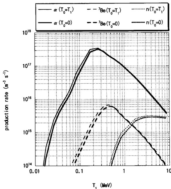
Fig. 4 Production rates of  $\alpha$  particle,  $^7\text{Be}$ , and neutron, from p-B reactions. For each particles, two extreme cases of  $T_0 = T_1$  and  $T_0 = 0$  are shown.
