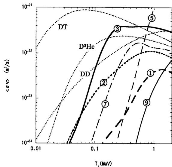
Fig. 3 Fusion cross-section as a function of ion temperature  $T_i$ . Number indicates reaction type and identical to the equation number in the article. Cross-sections of eqs. (4), (6) and (8) are small ( $< 10^{-25} \text{ m}^3/\text{s}$  at  $T_i < 2 \text{ MeV}$ ) and not illustrated.
