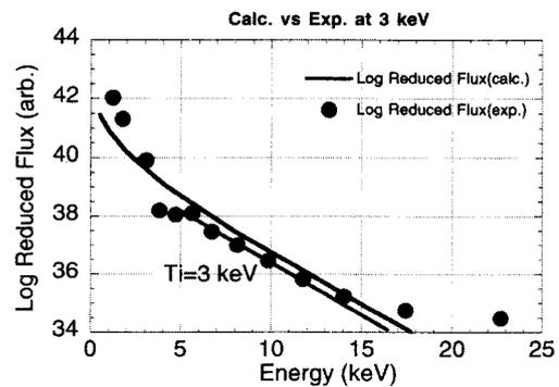
Fig. 3 Typical Energy spectrum at the NBI plasma. The straight line indicates the calculation results.
