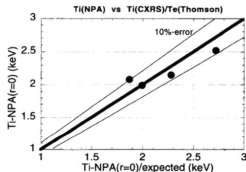
Fig. 4 The comparison of NPA with CXRS. Two straight lines shows the 10% errors.
