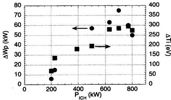
Fig. 5 The preliminary results of ICH heating. The stored energy and ion temperature increase by the ICH.
