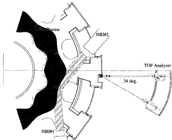
Fig. 1 The arrangement of NBI#1, #2 and analyzer. The analyzer can be scanned horizontally 35 degrees. NBI#1 and #2 are the co- and counter-injectors, respectively.
