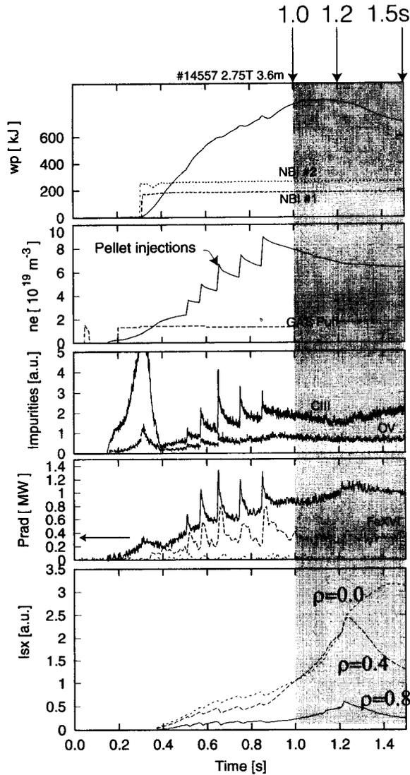
Fig. 5 Plasma parameters of # 14557. Impurity radiation profile is peaked in the hatched time window.
