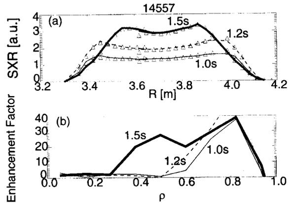
Fig. 6 SXR profile (a) and Enhancement factor profile (b) at 1.0 s, 1.2 s and 1.5 s in the plasma show in Fig. 5.
