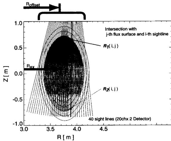
Fig. 1 Schematic view of the soft X-ray measurements in LHD.
