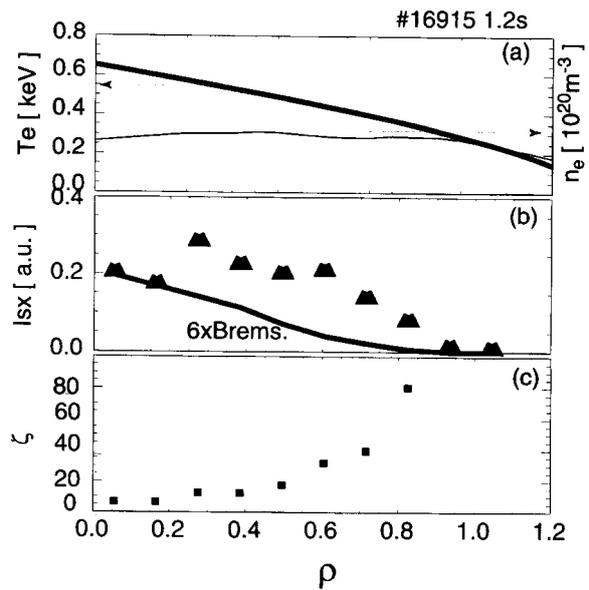
Fig. 4 Electron temperature and density profiles (a), reconstructed emissivity profile (triangles) and calculated bremsstrahlung profile (b) from  $T_e(\rho)$ ,  $n_e(\rho)$ , enhancement factor  $\zeta$ (c) are shown as a function of normalized minor radius  $\rho$ .
