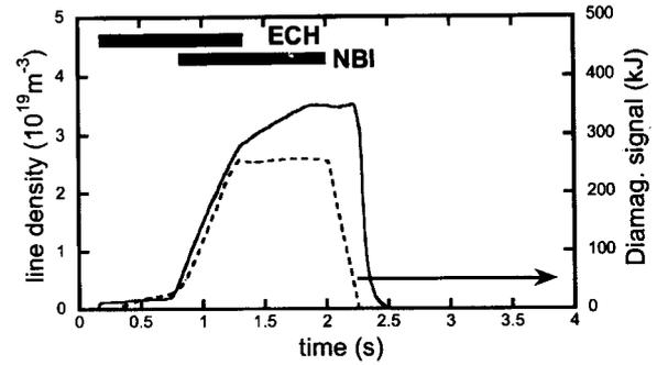
Fig. 2 Time evolution of the electron line density (solid line) and the plasma diamagnetism for the LHD combined heating plasmas; shot #12746 (dotted line).
