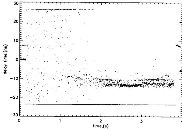
Fig. 5 Dual-polarized experiments, because of poor reflection with respect of pure O- or X-mode case timing system start to be triggered by noise (with timing about 26 ns), or not reflected backward (-23.5 ns); shot #13771.
