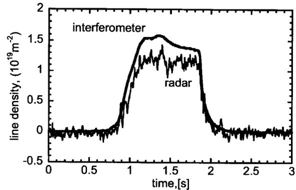
Fig. 6 Delayometry type of operation. A comparison of line integral density obtained by means of interferometry and a pulse radar system. Reflectometry raw data was smoothed within 15 points; shot #12694.
