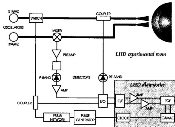
Fig. 1 The block diagram of the LHD U-band pulsed radar reflectometer.
