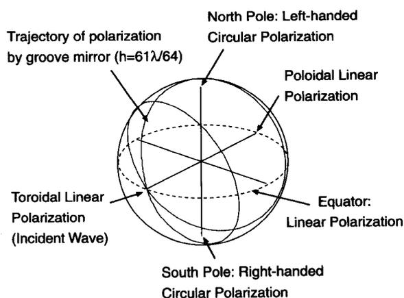
Fig. 4 Trajectory of the polarization produced by rotating a single grooved mirror (groove depth  $=61/64\lambda$ ) for Fig. 3 on the normalized Poincaré sphere.
