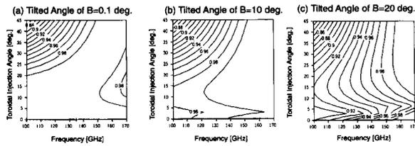
Fig. 5 Contour of the O-mode purity produced by a single mirror polarizer ( $h = 0.341$  mm,  $c = d/2 = 0.5$  mm). The tilted angles of magnetic field line are  $0.1^\circ$  in 5(a),  $10^\circ$  in 5(b) and  $20^\circ$  in 5(c).
