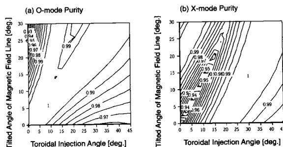
Fig. 3 Mode purities by a deep grooved polarizer ( $h = 61/64\lambda$ ) at 110 GHz. 3(a) O-mode purity and 3(b) X-mode purity.
