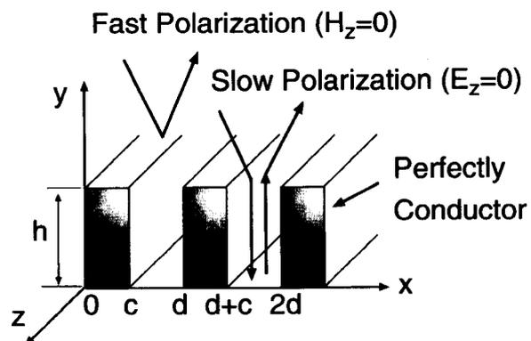
Fig. 1 Groove surface of a polarizer in rectangular coordinate system.
