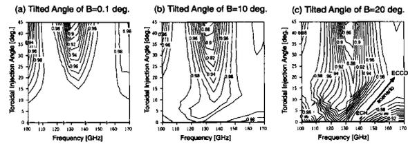
Fig. 6 Contour of the O-mode purity produced by a single mirror polarizer ( $h = 2.73$  mm,  $c = d/2 = 0.5$  mm). The tilted angles of magnetic field line are  $0.1^\circ$  in 6(a),  $10^\circ$  in 6(b) and  $20^\circ$  in 6(c).
