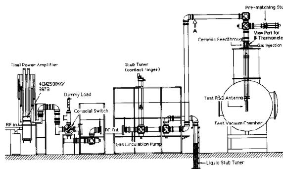
Fig. 3 Layout of ICRF test stand for R & D experiments of RF components.
