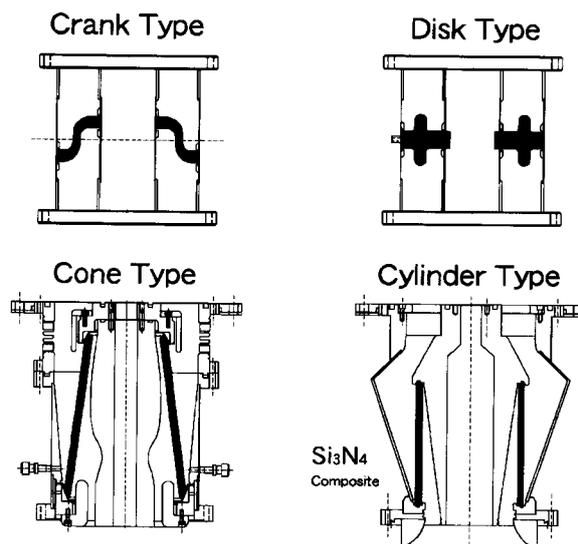
Fig. 5 Cross section of tested feedthroughs. Ceramic part is painted over with black.
