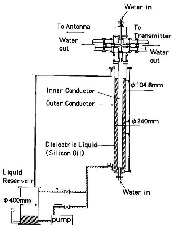
Fig. 4 Schematic drawing of liquid stub tuner.
