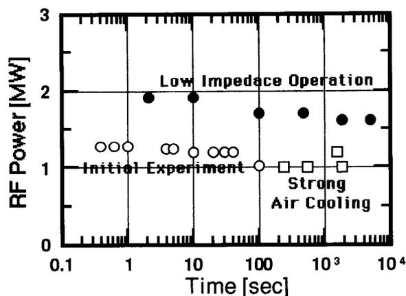
Fig. 2 Expansion of RF output power and duration time of the transmitter.
