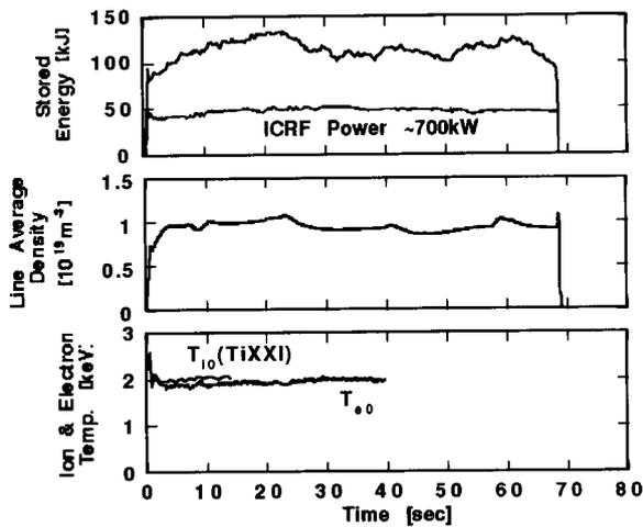
Fig. 6 Time evolution of plasma parameters during 68 seconds operation.
