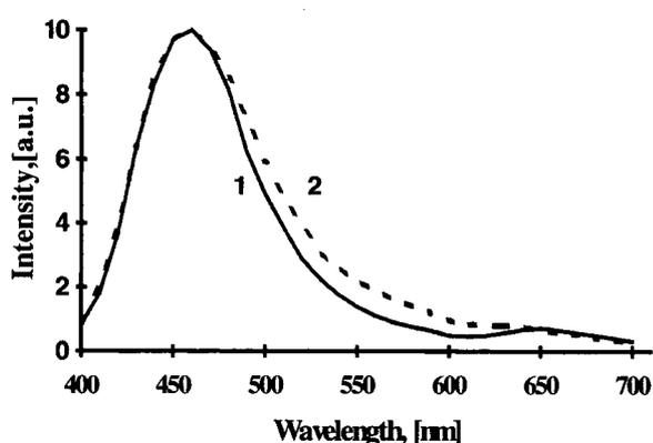
Fig.1 The ionluminescence spectra of  $\text{SiO}_2$  under proton bombardment: curve 1 - nonirradiated sample, curve 2 - the sample irradiated with absorbed proton doses of  $3 \times 10^{21}$  particles/cm<sup>3</sup>.
