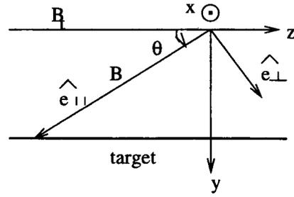
Fig. 1 The geometry of the region, magnetic field  $\mathbf{B}$  is in the  $y$ - $z$  plane, making an angle  $\theta$  with the toroidally continuous target surface.
