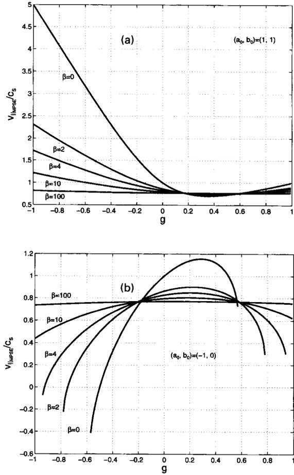
Fig. 2 The value of  $v_{\parallel MPSE}/c_s$  plotted vs. the strength of  $E \times B$  drift velocity  $g$ , for the values of  $\beta = 0.0, 2, 4, 10$  and  $100$ . Two cases presented are (a)  $(a_0, b_0) = (1, 1)$  and (b)  $(a_0, b_0) = (-1, 0)$ .
