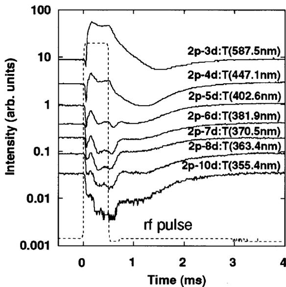
Fig. 2 Time evolution of the line emission intensities from principal quantum number  $n'$  from 3 through 10 in a fairly detached plasma at  $P \sim 5.85$  mtorr.
