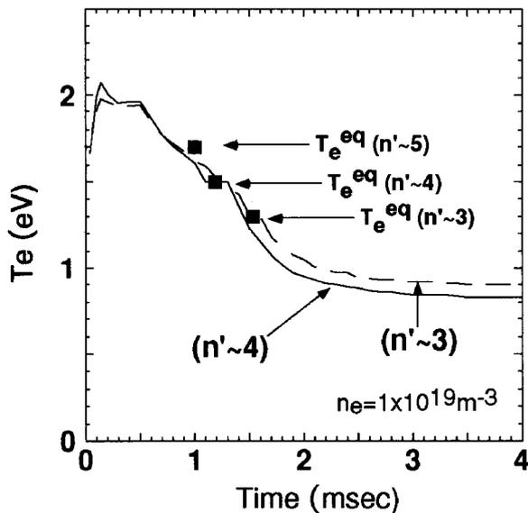
Fig. 4 Reconstructed time evolution of the electron temperature from the numerical results shown in Fig. 3.
