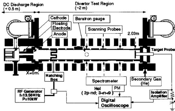
Fig. 1 Schematic of the experimental apparatus, NAGDIS-II.
