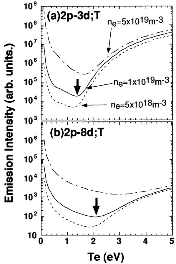
Fig. 3 Dependence of line emission intensities from principal quantum number  $n' \sim 3$  and 8 on the electron temperature calculated by CR model as a parameter of plasma density.
