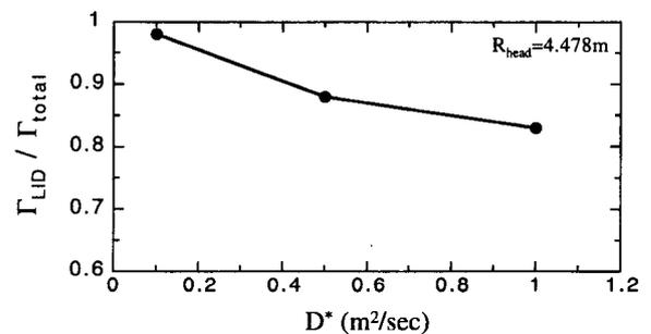
Fig. 3 Collecting efficiency of particles by LID.  $\Gamma_{\text{total}} = \Gamma_{\text{LID}} + \Gamma_{\text{HD}}$ , where  $\Gamma_{\text{LID}}$  and  $\Gamma_{\text{HD}}$  are particle flux to LID head and helical divertor, respectively.
