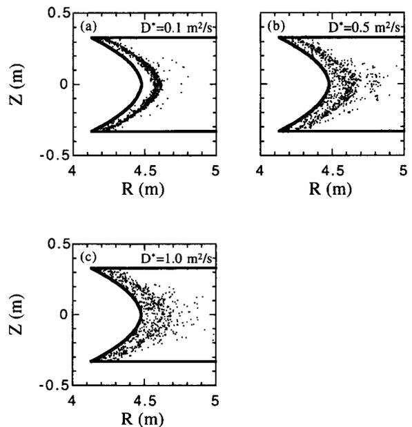
Fig. 2 Striking point patterns on LID head for (a)  $D^* = 0.1$ , (b)  $0.5$  and (c)  $1.0 \text{ m}^2/\text{sec}$ , respectively.
