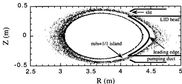
Fig. 1 Schematic of LID. Diffused particles are directed to the LID head along the island periphery, detouring to avoid the leading edge.
