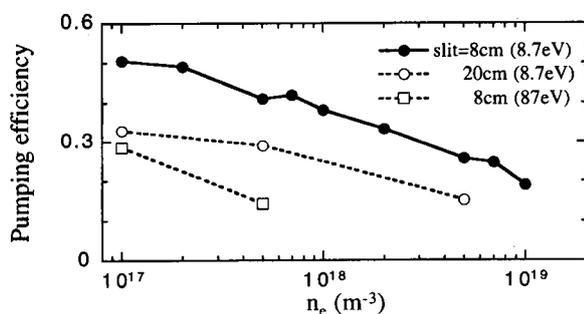
Fig. 4 Pumping efficiency of LID for different slit size and temperature.
