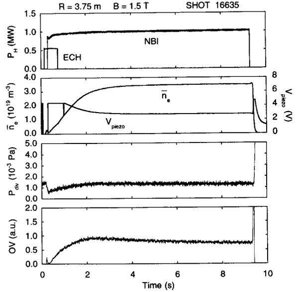
Fig. 4 Typical long pulse discharge with carbon divertor plates. The plasma density is feedback controlled by the gas puffing system. The amount of gas injection decreases with time and is kept almost constant at the end of discharge.
