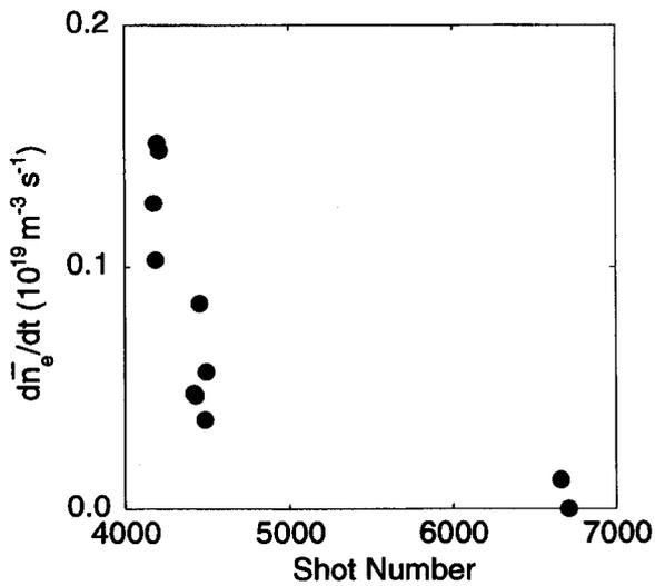
Fig. 1 Effect of wall conditioning on long pulse operation. The increase rate of plasma density is estimated at about 5 s and decreases with the number of plasma discharge because of daily wall conditioning (He glow, Titanium gettering).
