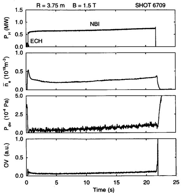
Fig. 2 Quasi-steady-state discharge with stainless steel divertor plates. There is no external gas puffing during NBI heating. This type of discharge is restricted in low density regime.
