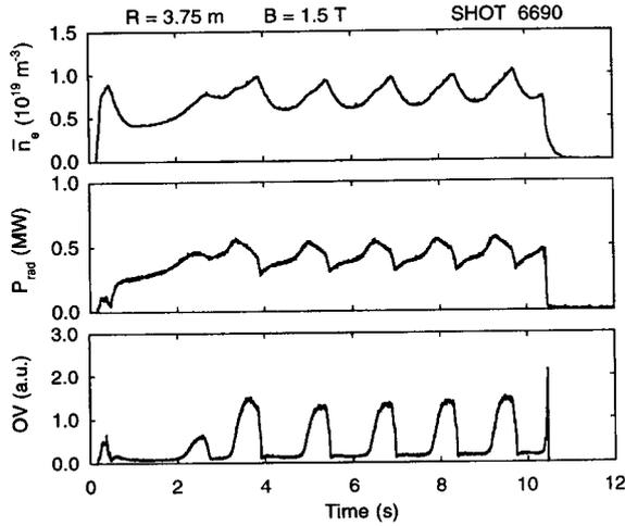
Fig. 3 Long pulse discharge with a slow relaxation oscillation. Gas puffing is also performed only in the rising phase of plasma density but the amount is little more than that in Fig. 2.
