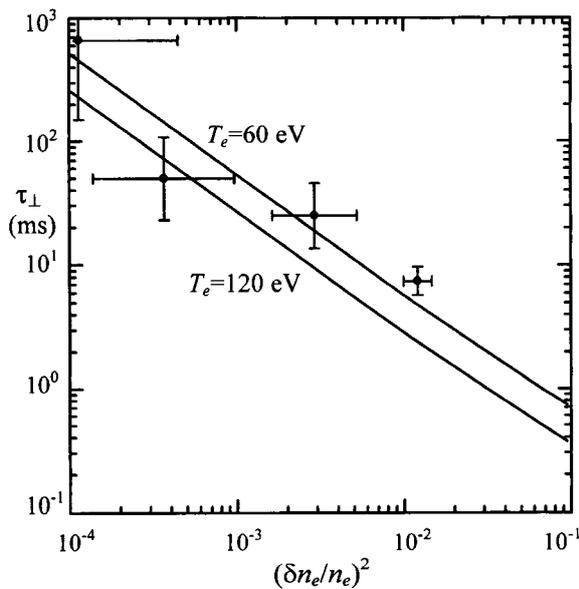
Fig. 1 Radial confinement time for GAMMA-10 plasma calculated using Eq. 7 (solid lines) and in experiments [13] (points).  $B = 0.4$  T,  $a = 0.2$  m,  $T_e = 60..120$  eV.
