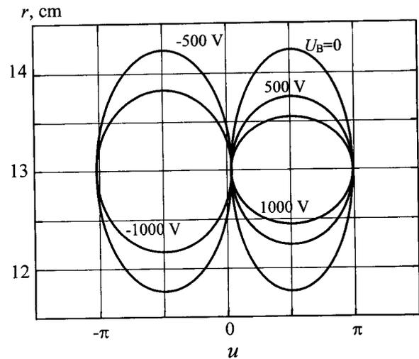
Fig. 2 Particle oscillations under the influence of single mode perturbation. The electric field amplitude is 30 V/m, resonant radius is 0.13 m,  $B = 0.4$  T,  $a = 0.2$  m,  $T_e = 100$  eV.
