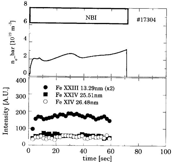
Fig. 6 (a) Time evolution of  $n_{e\bar{}}$ , (b) Time evolution of line intensity from highly-ionized iron at the core or the middle on long-pulse NBI discharge.
