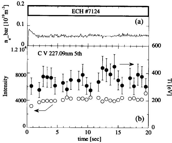
Fig. 4 (a) Time evolution of  $n_{e\bar{}}$ , (b) Time evolution of  $T_i$  and line intensity on long-pulse ECH discharge.
