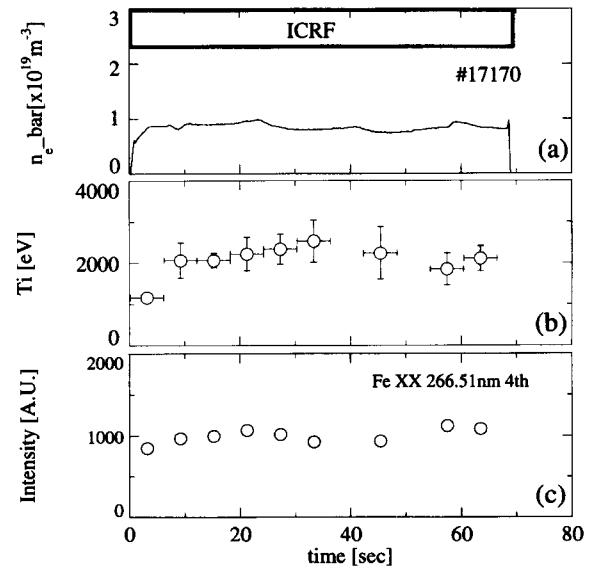
Fig. 2 (a) Time evolution of line-average electron density  $n_e$ , (b) Time evolution of Doppler ion temperature  $T_i$  from Fe XX, (c) Time evolution of line intensity of Fe XX spectrum in long-pulse ICH discharge.
