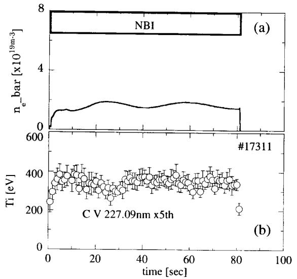
Fig. 5 (a) Time evolution of  $n_{e\bar{}}$ , (b) Time evolution of  $T_i$  from C V on long-pulse NBI discharge.
