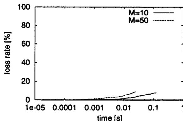
Fig. 3 Monte Carlo calculation of Alpha particle confinement.  $M$  denotes the number of Boozer spectrum modes used in the calculation.
