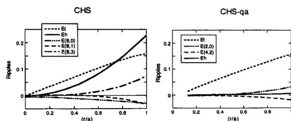
Fig. 1 Comparison of Boozer spectrum for CHS and CHS-qa. Mode numbers in the bracket are for toroidal and poloidal modes.  $E_t$  is toroidicity and  $E_h$  is main helical ripple.
