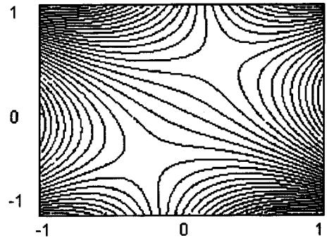
Fig. 3 Structurally stable magnetic configuration with two  $X$ -lines.
