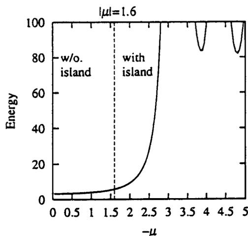
Fig. 2 Magnetic energy versus  $\mu$  of the Taylor state given by Eq.(1). For  $|\mu| > 1.6$ , a magnetic island appears.
