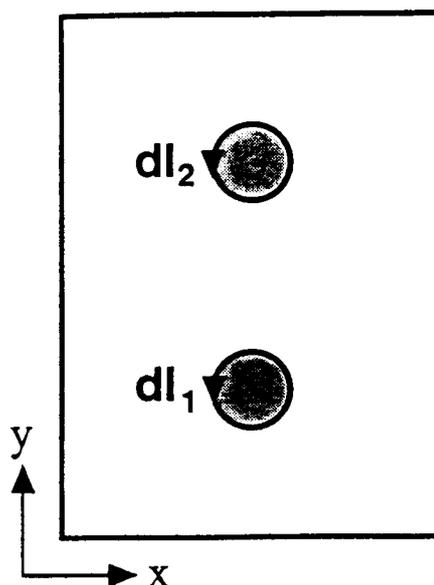
Fig. 1 A schematic plot of MRX configuration showing a path of integration defined in Eq.(2). Shaded regions indicate cross-sections of flux-core coils.
