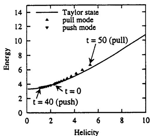
Fig. 3 Evolution of the magnetic energy and helicity found in MHD simulations for "pull" and "push" modes. Solid line shows the Taylor state. Marks representing simulation results are plotted at every  $5 \tau_A$ .
