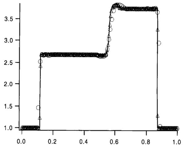
Fig. 2 The results of check MHD test simulations for the numerical scheme with an artificial wind. The test is described in [4] and in papers cited there. Line - 400 cell per the full length (limiter with  $\beta = 1.3$ , triangles - 200 cells ( $\beta = 1.4$ ), circles - 100 cells ( $\beta = 1.7$ ). The time step corresponds to the CFL number  $\sigma = 0.8$
